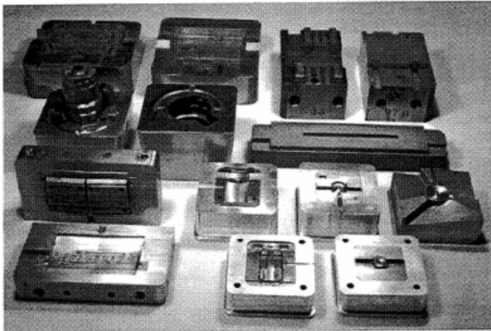
Figure 2. A set of tooling inserts printed for various industrial applications. All tools have been infiltrated and approximately half of the tools have been finished and used to inject parts. For scale, the tool in the lower left hand corner is 6” long.
