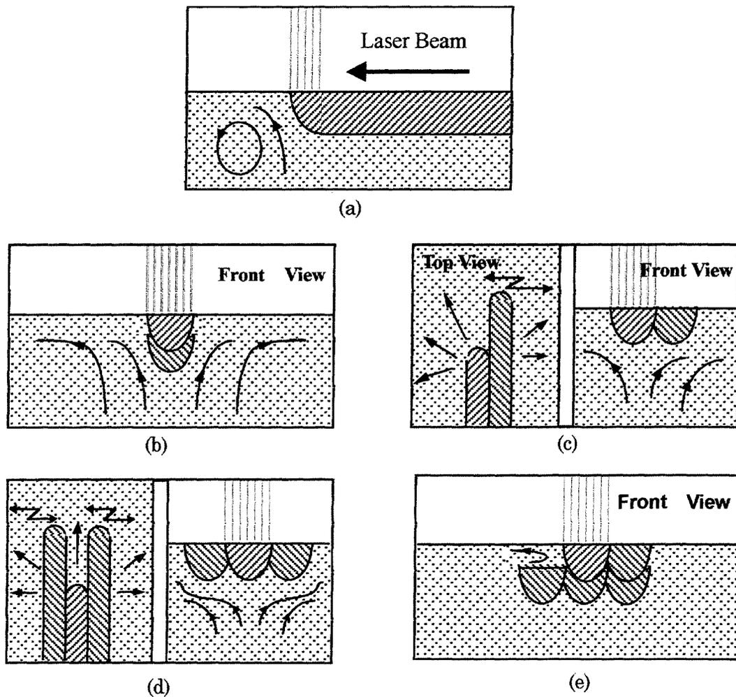
Figure 3 Flow Behavior of Photopolymer during Laser Scanning
