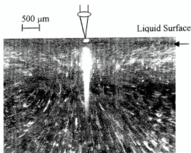
Figure 2 Partial Flow of Liquid Photopolymer During Laser Exposure
