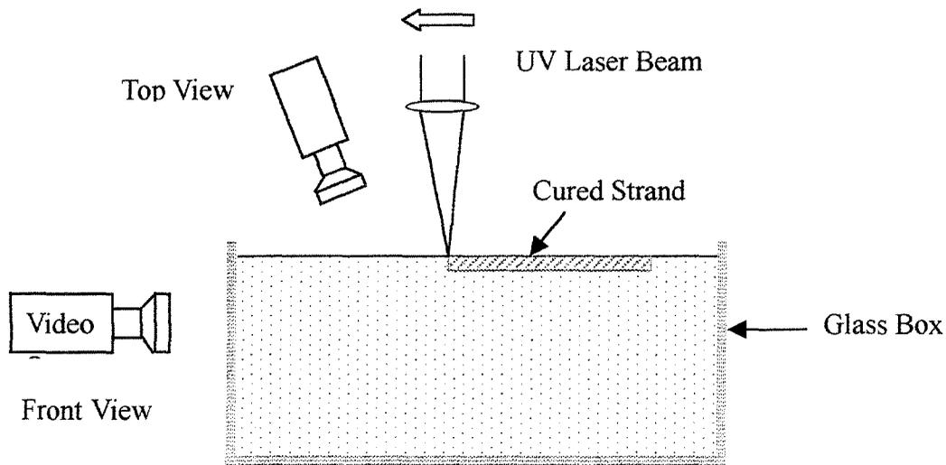
Figure 1 Observation of Flow during Laser Exposure
