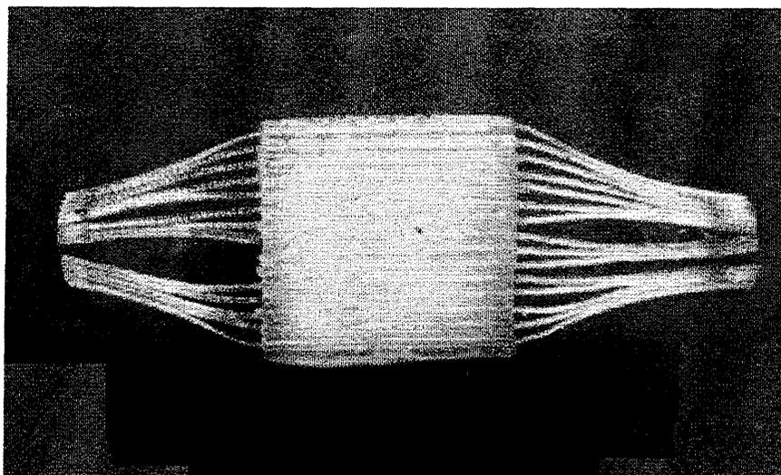
Figure 7 Connected Free Ends of Continuous Cured Strands
