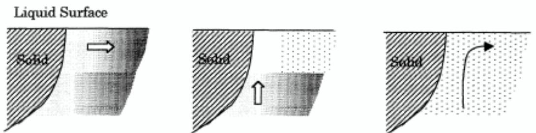
Figure 10 Enlarged Schematic Side View of Partial Microscopic Flow of Photopolymer during Laser Exposure
