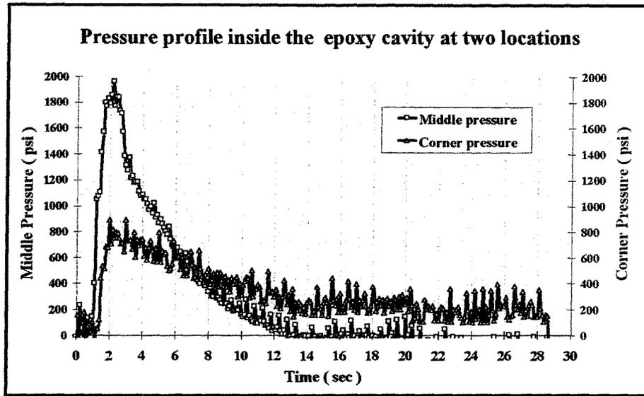
Figure 6. The pressure profile inside the cavity at the centre and after the cube
