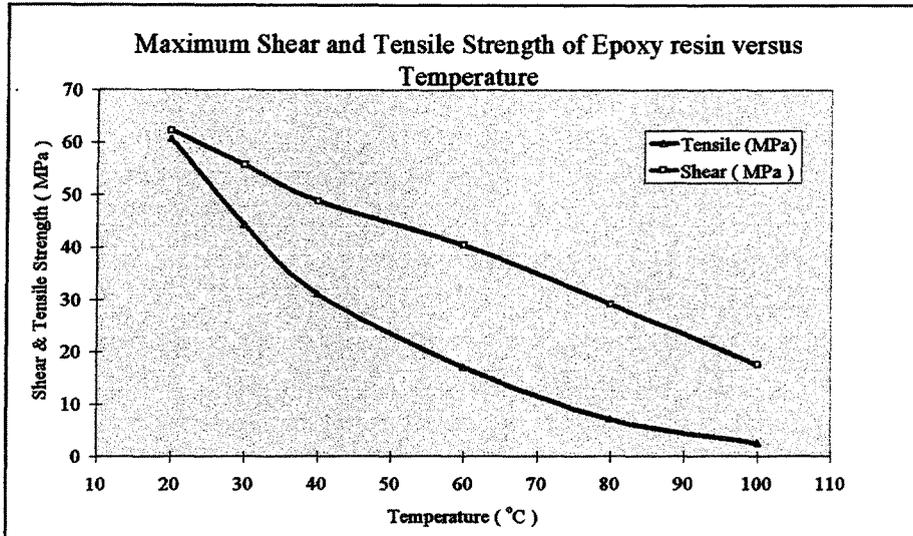
Figure 4. Maximum Tensile & Shear strength of epoxy SL5170 versus temperature
