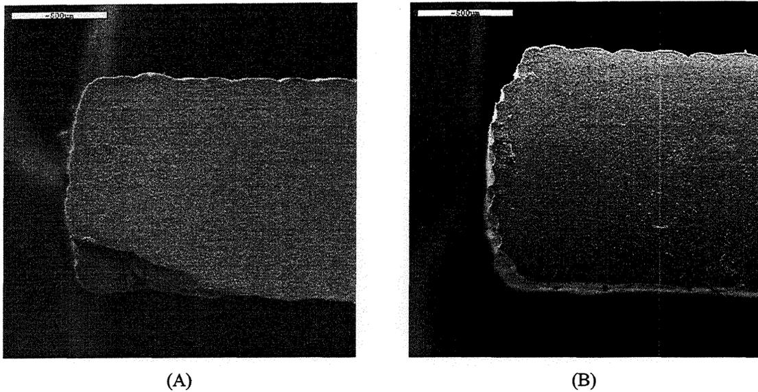
**Figure 7.** Cross sections of alumina parts printed displaying the effect of layer height on the surface finish of the parts. Parts with 50  $\mu\text{m}$  layer height (A) has smoother surface finish than parts printed with 100  $\mu\text{m}$  layer height (B). Binder concentration is identical for both parts. (Scale marker bar is 500  $\mu\text{m}$ )
