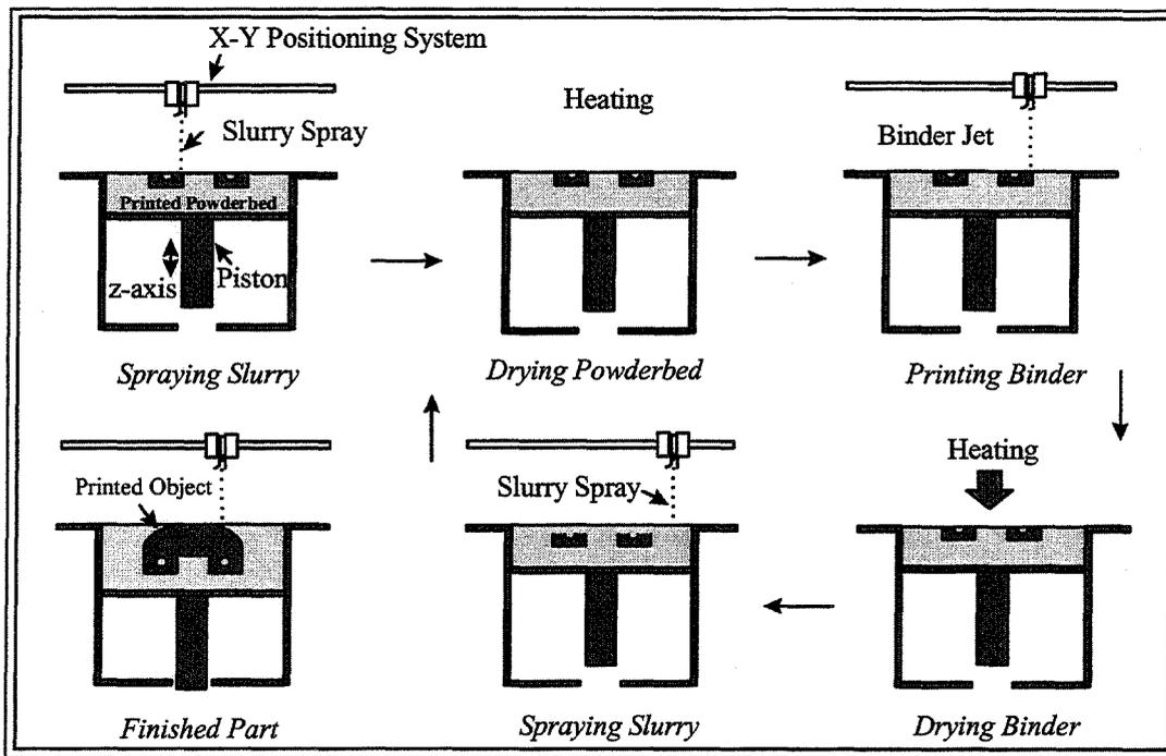
Figure 1. Schematic of the slurry-based 3DP process
