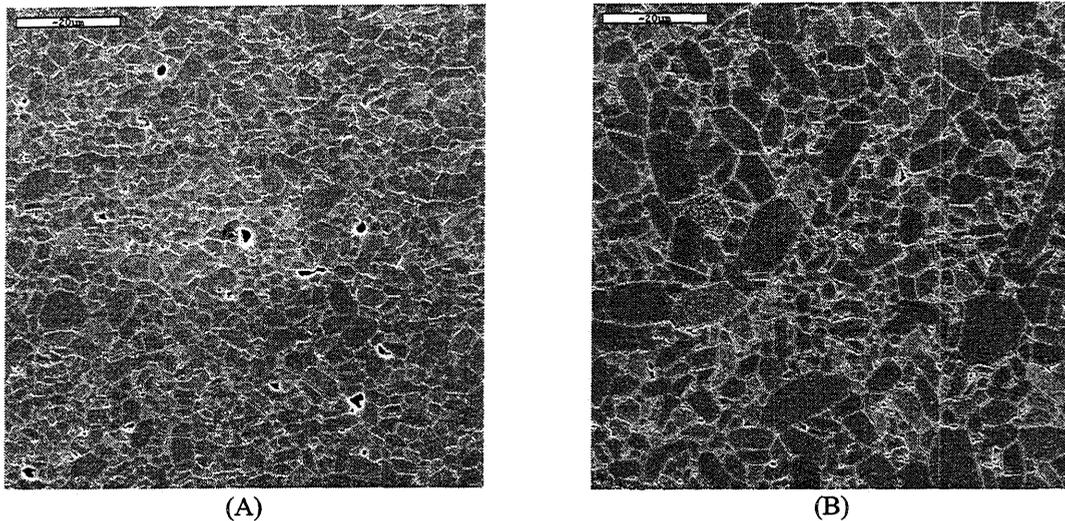
**Figure 2.** Polished cross-sections of samples sintered at 1650°C. Microstructure of slurry-based 3DP parts (A) are similar to powder beds prepared by slip casting (B). (Scale marker bar is 200 μm).
