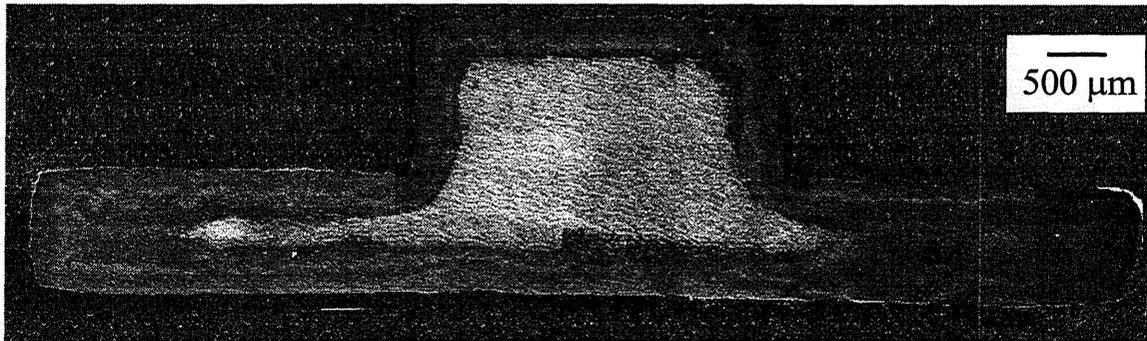
**Figure 10.** A cross section of a bisque fired silicon nitride part shown in Figure 9. The material with different contrast near the surface of the sample is the result of mounting material only partially permeating the porous sample.
