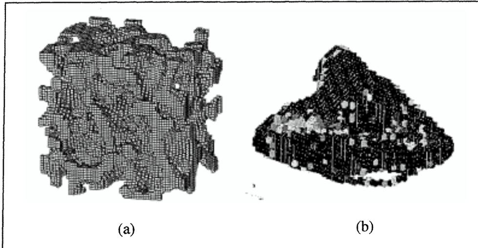
**Figure 2.** Examples of image data that can be input to the Solid Builder module (a) segmented CT data of bone microstructure (b) finite element model of a suspension arm
