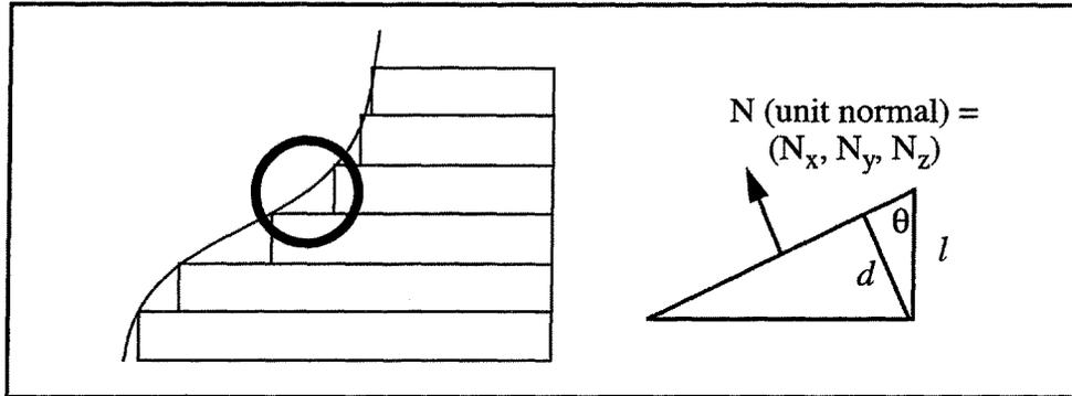
**Figure 3.** Illustration of cusp height ( $d$  is cusp height,  $l$  is layer thickness)
