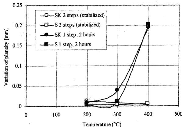
Figure 4: Variation of planarity due to the second step heat treatment after a first stabilization treatment (2 hours at 600 °C).
