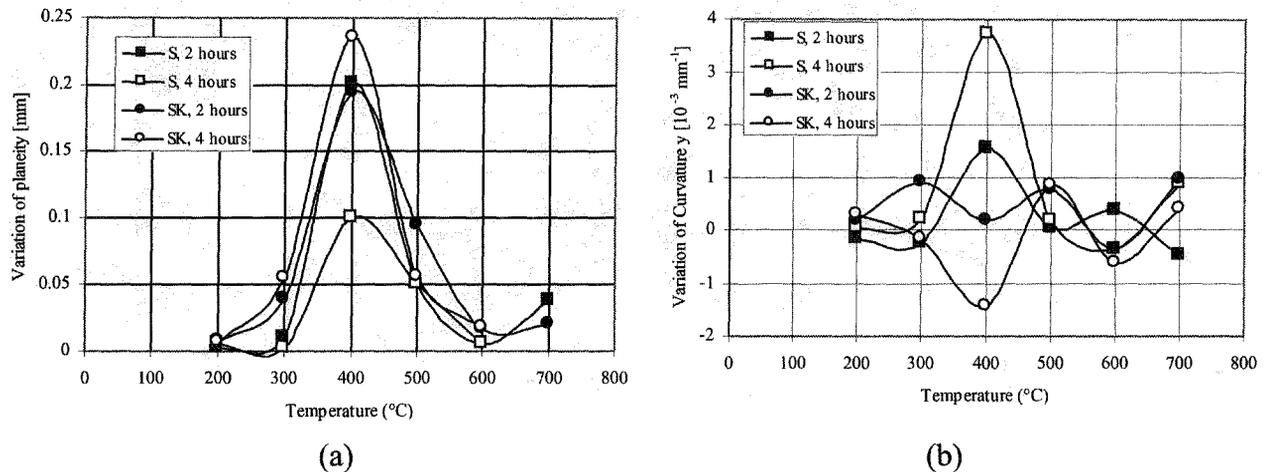
Figure 3: variations of (a) planarity and (b) curvature in the y direction, as a function of the treatment temperature, for the different treatment durations and strategies.
