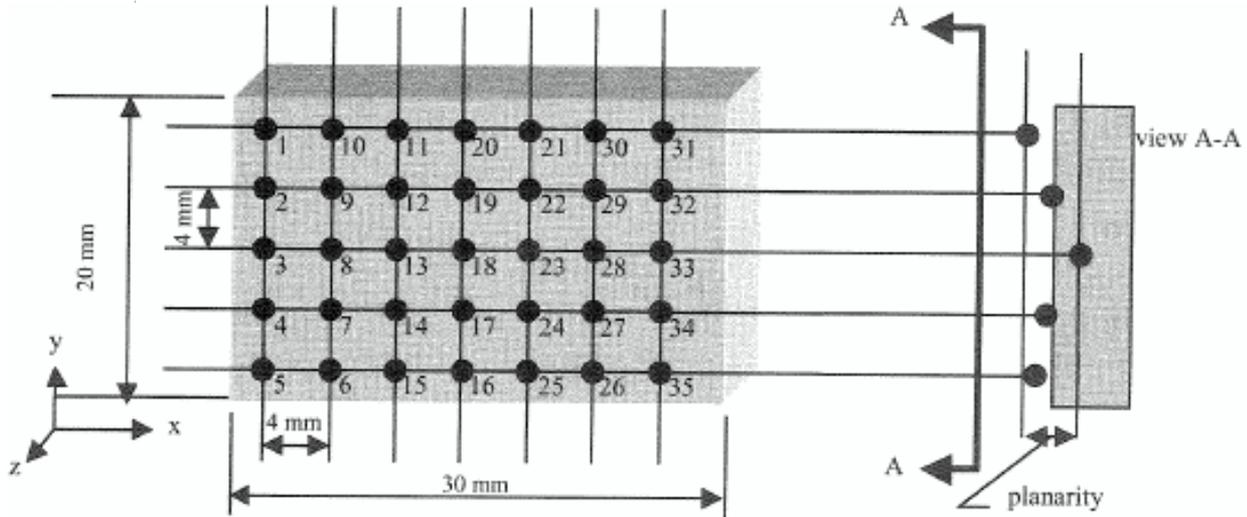
Figure 2: measurement locations at the sample surface and definition of planarity.
