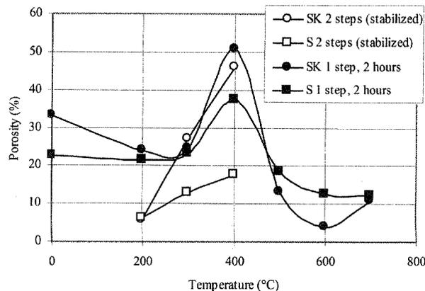
Figure 6: effect of a stabilization heat treatment (2 hours at 600 °C) on the porosity.
