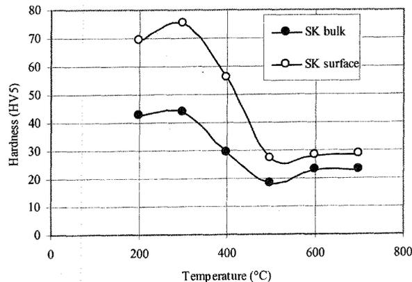
Figure 8: surface and bulk hardness (measured in the middle of the sample), for SK specimens.
