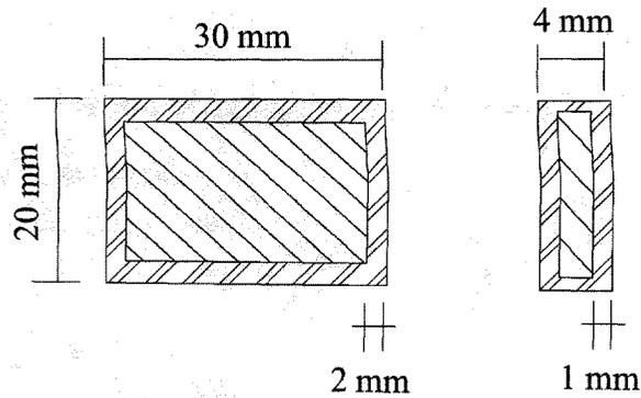
Figure 1: schematic of the SK samples, with skin depths.
