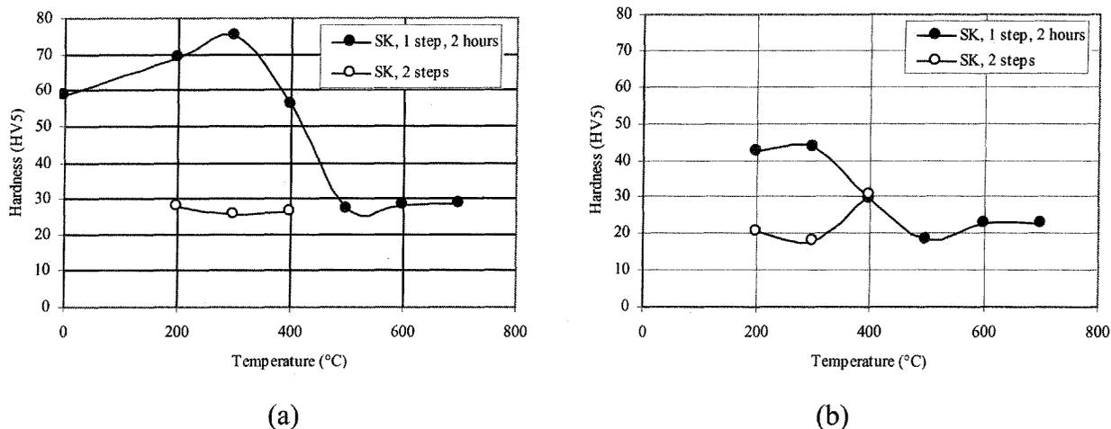
Figure 9: (a) surface and (b) bulk hardness for the one-step samples and after the two-step treatment (stabilization).
