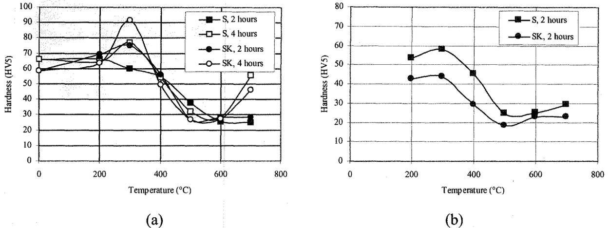
Figure 7: (a) surface hardness as a function of treatment temperature, for different treatment times. (b) Bulk hardness of the one-step samples treated 2 hours, measured in the cross-section.
