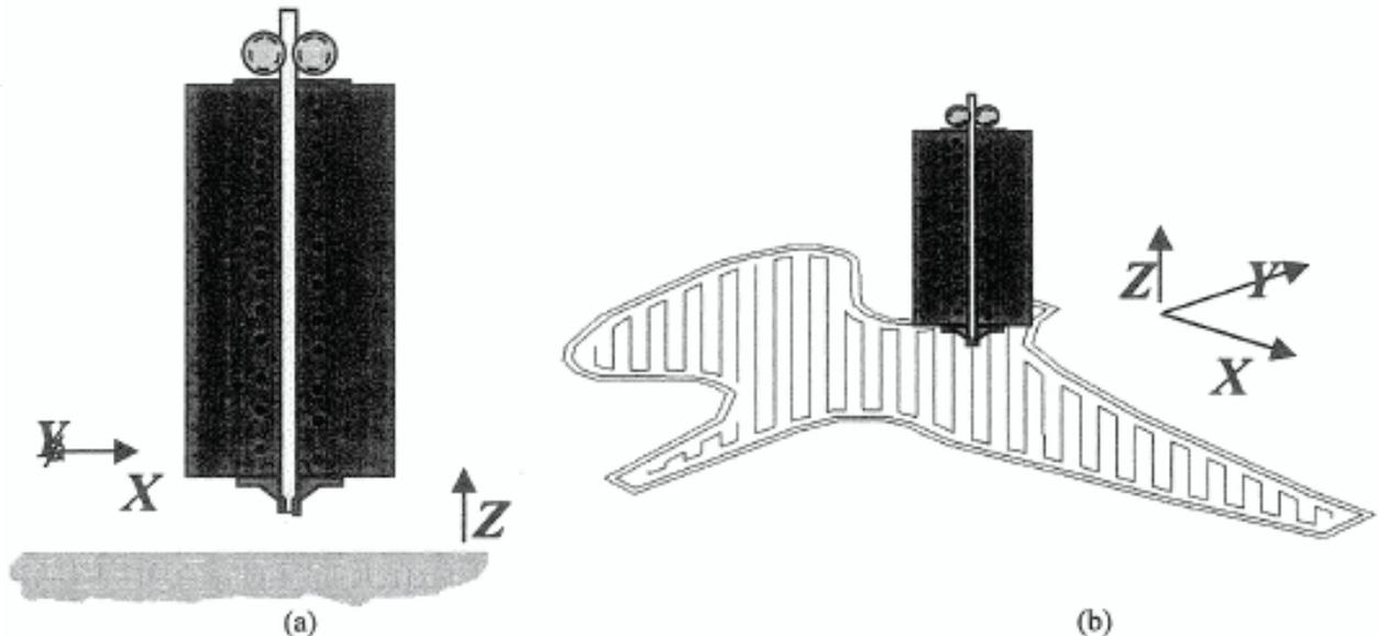
**Figure 1: Schematic of the Fused Deposition (FD) process.** To the left (a) is a close up of a straightened liquefier, showing the material being deposited on a flat platen to form the part. At right (b), the tool is shown traversing a path that describes the cross section of the part.
