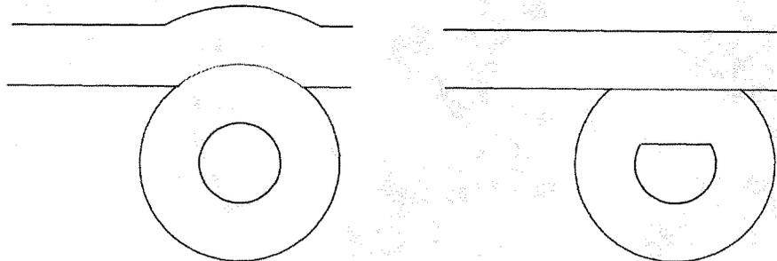
**Figure 4: Two options of the new toolpath giving the designer control over feature retention. On the left the circularity of the hole is preserved, while on the right the fin surface is preserved.**
