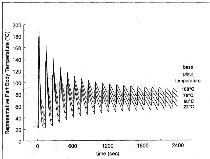
**Figure 3:** Parametric variation of base plate temperature: simulated, dynamic temperature profiles inside a 20-layer SiC LOM part during the building process (120 seconds per layer) using the parameters given in Table 2 (trial 3, 5, 6, 7).
