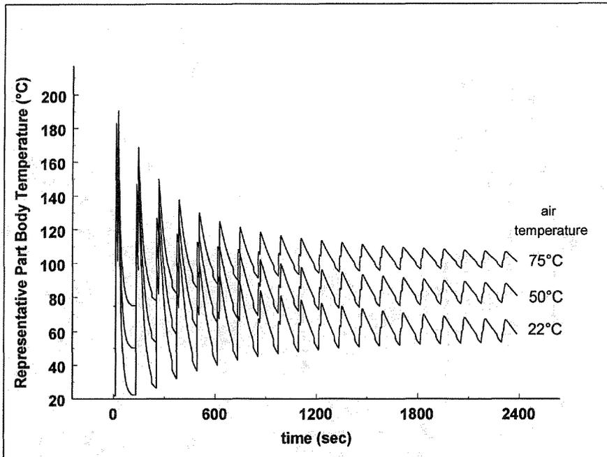
**Figure 4:** Parametric variation of chamber air temperature: simulated, dynamic temperature profiles inside a 20-layer SiC LOM part during the building process (120 seconds per layer) using the parameters given in Table 2 (trials 3, 8, 9).
