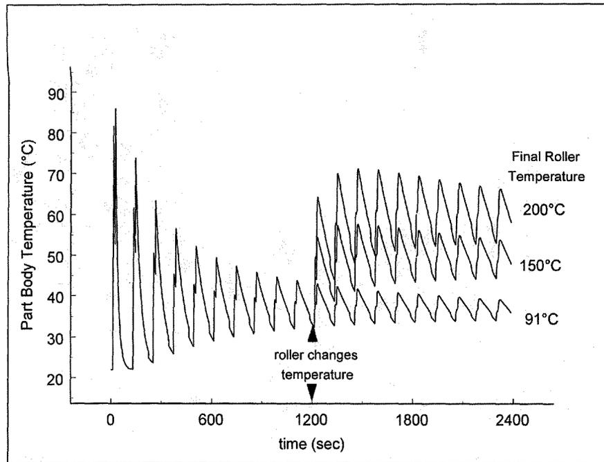
**Figure 6:** Effect of changing the roller temperature (from 91°C) halfway through a run: simulated, dynamic temperature profiles inside a 20-layer SiC LOM part during the building process (120 seconds per layer) using the parameters given in Table 2 (trials 17, 18).
