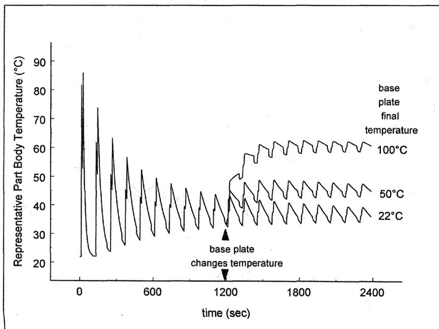
**Figure 5:** Effect of changing base plate temperature halfway through a run: simulated, dynamic temperature profiles inside a 20-layer SiC LOM part during the building process (120 seconds per layer) using the parameters given in Table 2 (trials 15, 16).
