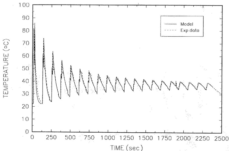
**Figure 1:** Base simulation and experimentally measured temperature profile for a 20-layer, SiC LOM part, as measured by a thermocouple just above the 0<sup>th</sup> layer (foam tape base) during the build process [9]. The cycle time is 120 seconds per layer. The experimental conditions are given in Table 1 and Table 2 (trial #1).
