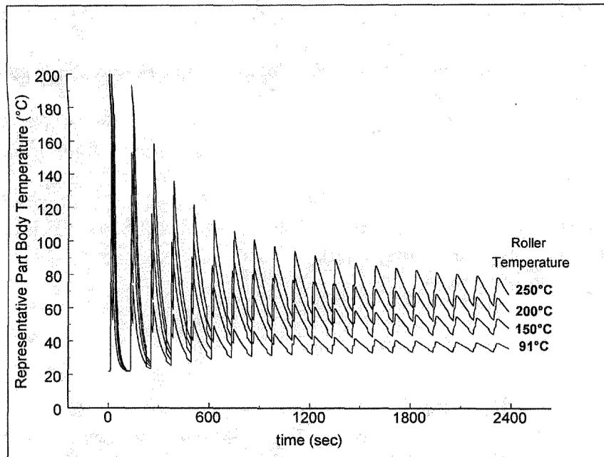
**Figure 2:** Parametric variation of roller temperature: simulated, dynamic temperature profiles inside a 20-layer SiC LOM part during the building process (120 seconds per layer) using the parameters given in Table 2 (trials 1-4).
