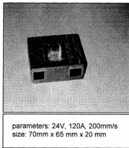
**Fig. 5:** Solid test part
