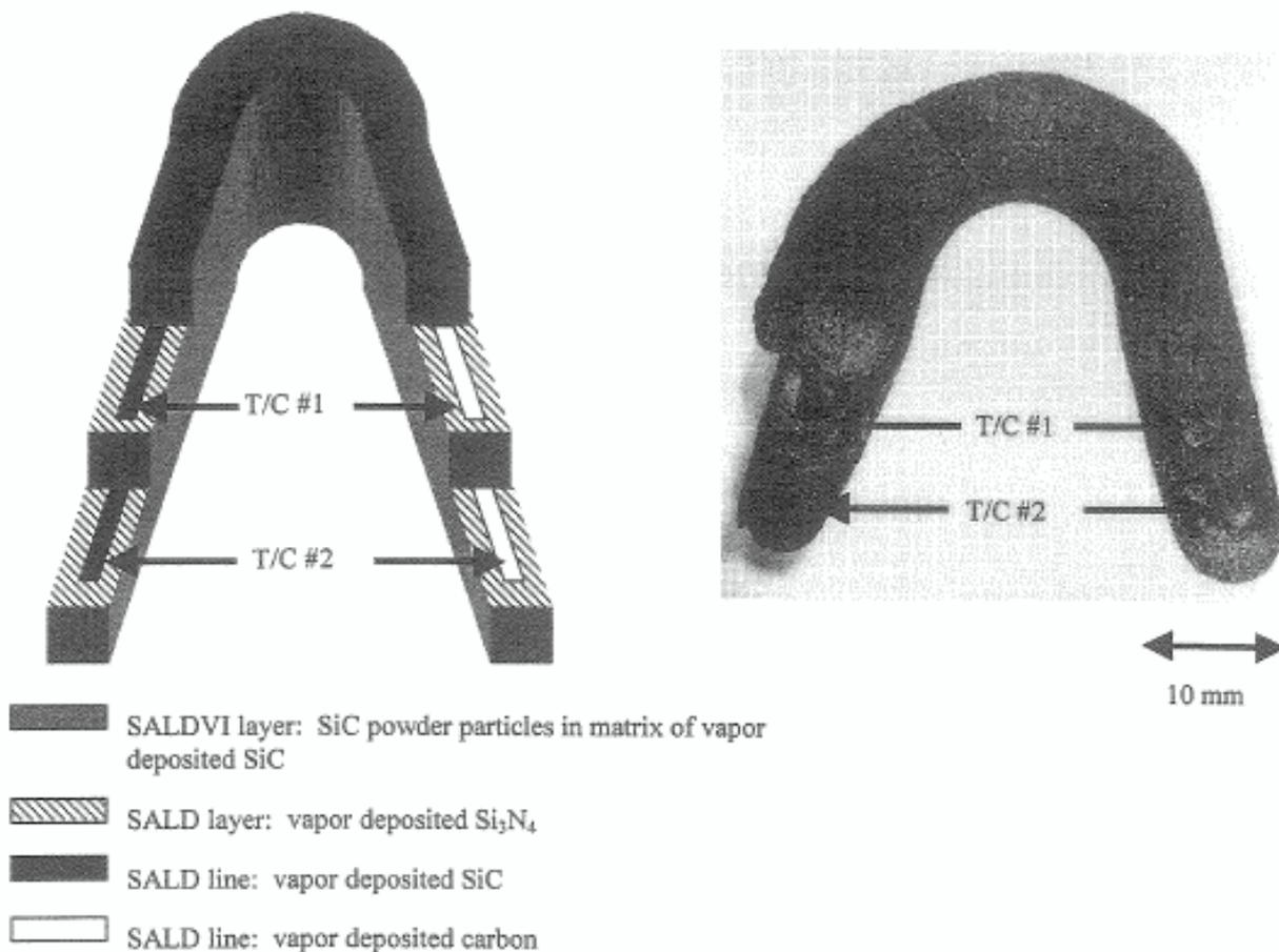
Figure 2. Bulk SiC shape containing two embedded SiC/C thermocouples
