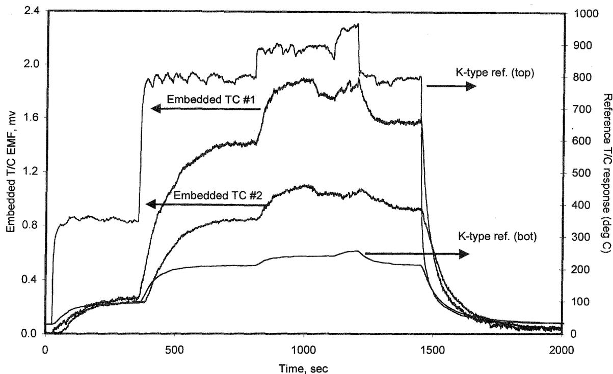
Figure 3. Response of embedded SiC/C thermocouples to an applied temperature history
