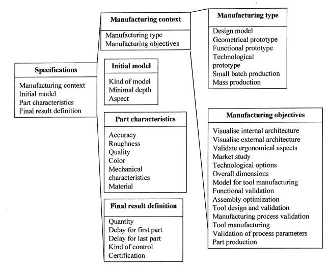
Figure 1. Some elements of specifications decomposition
