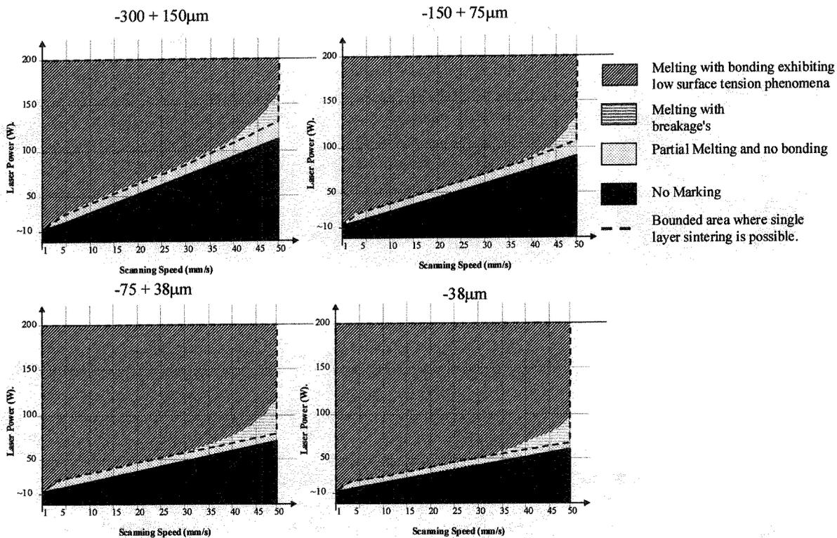
Figure 8: Sintering maps for 314S processed within an argon atmosphere.
