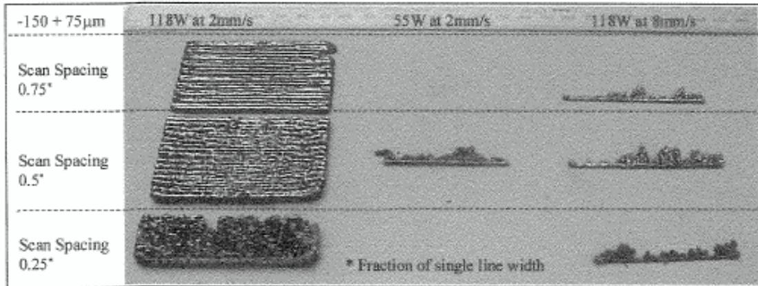
Figure 4: Examples of air atmosphere sintering.
