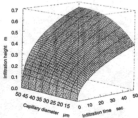
**Figure 3: Calculated silicon infiltration height**
