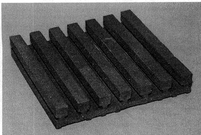
**Figure 8: Test bars for bending tests with support**
