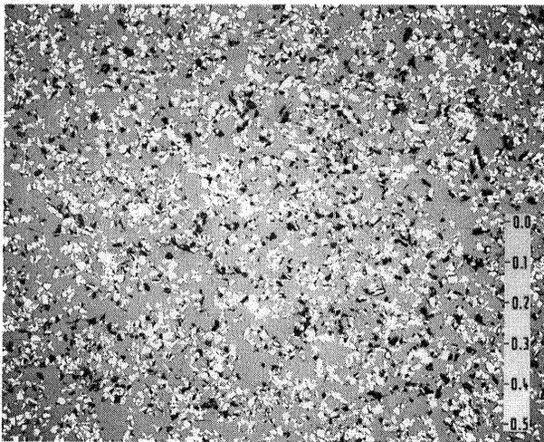
**Figure 6: Green part structure infiltrated with phenolic resin**
