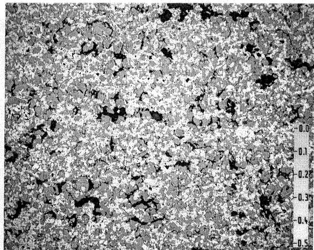
**Figure 7: Final structure of a polysilazane infiltrated sample after pyrolysis**
