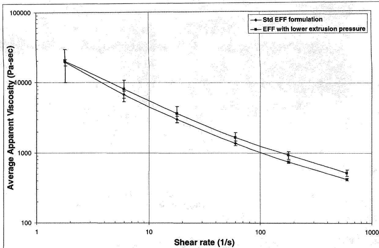
Figure 7. Comparison of shear rate-viscosity behavior of EEA binder formulations with 55 vol%  $\text{Si}_3\text{N}_4$  with and without an acryloid addition, at 150°C.
