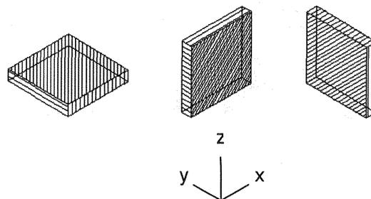
Figure 1: Sample Orientation for Thermal Expansion Measurements
