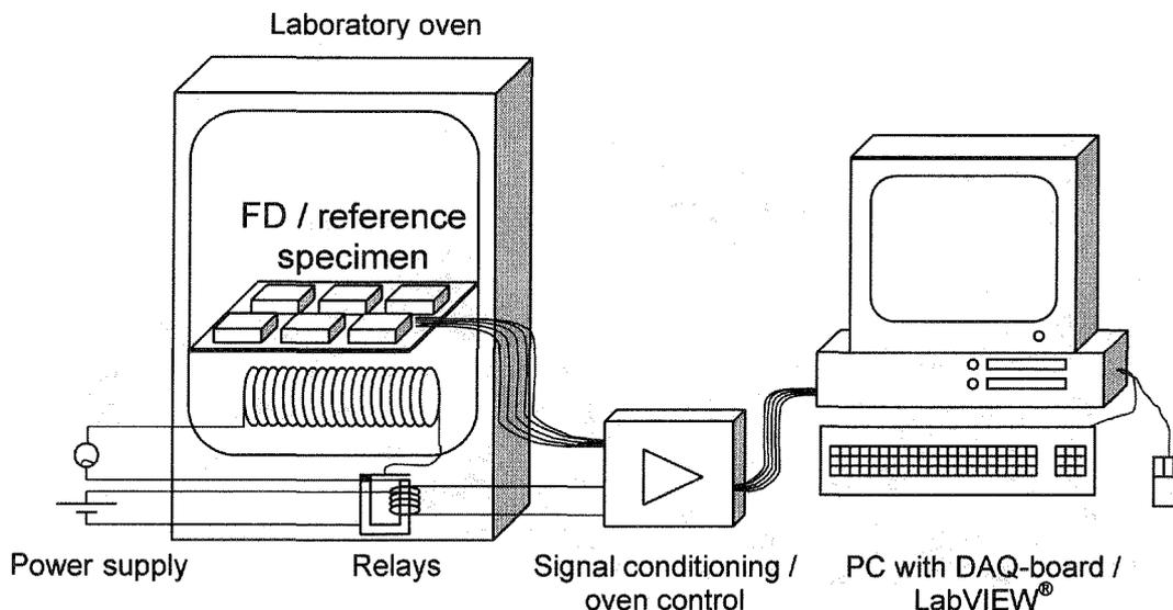
**Figure 2:** Experimental set-up for thermal expansion measurements
