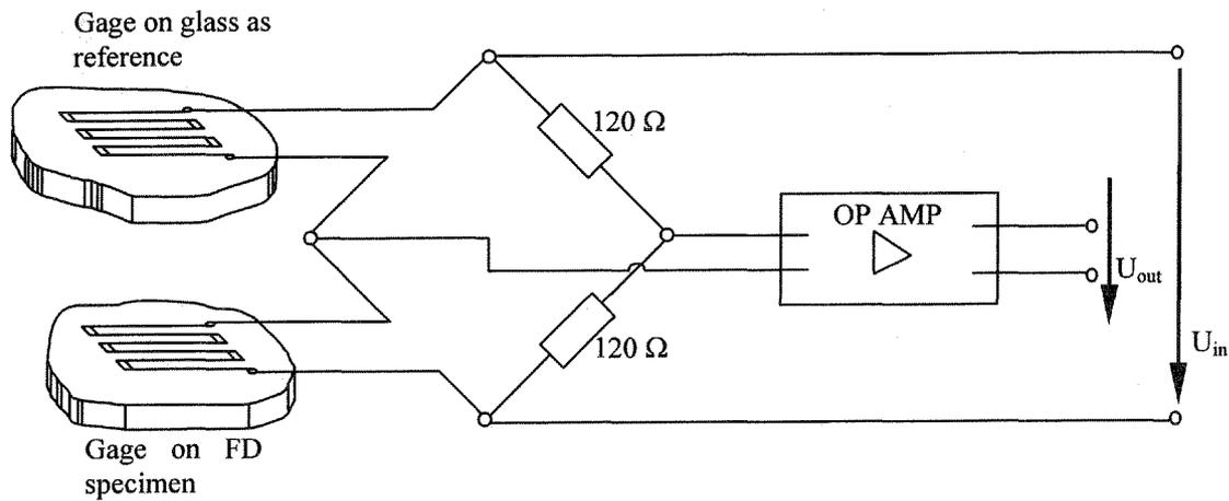
**Figure 3:** Half bridge circuit for strain measurements
