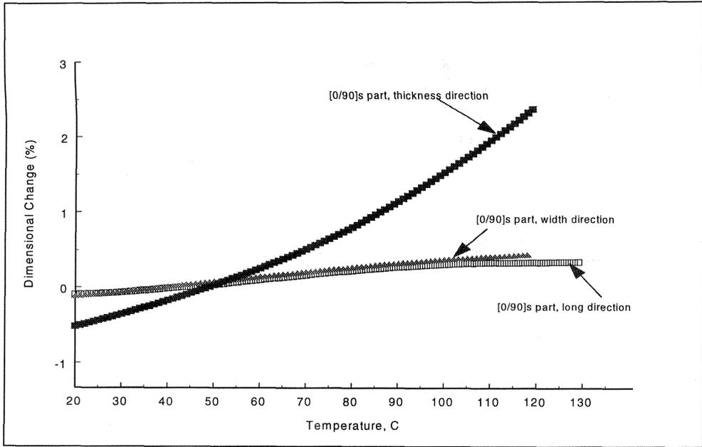
**Figure 3.** Comparison of N1 linear thermal expansion as a function of part orientation for [0/90]s part.
