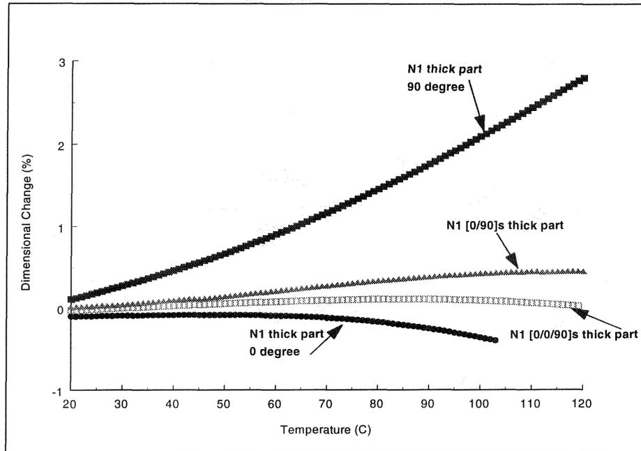
**Figure 4.** Comparison of the thermal expansion properties of N1 thick parts.
