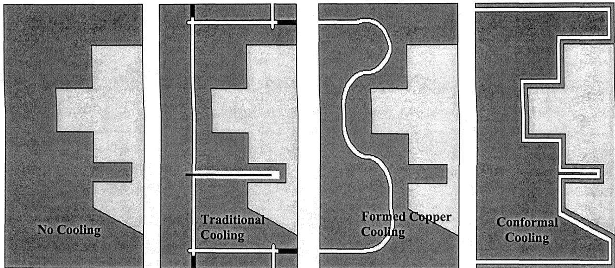
**Figure 2. Cooling Configurations**
