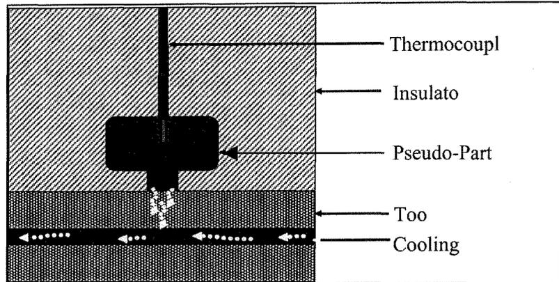
Figure 4. Test Cell Design
