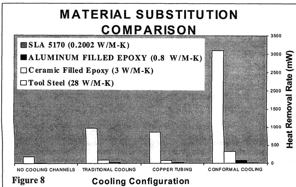
challenging to transfer heat through. Ceramic filled epoxy<sup>7</sup> is a significant improvement over aluminum filled epoxy while tool steel is even a greater improvement over the ceramic filled epoxy. Figure 9 illustrates the addition of aluminum and copper to figure 8, again a significant improvement over tool steel.
