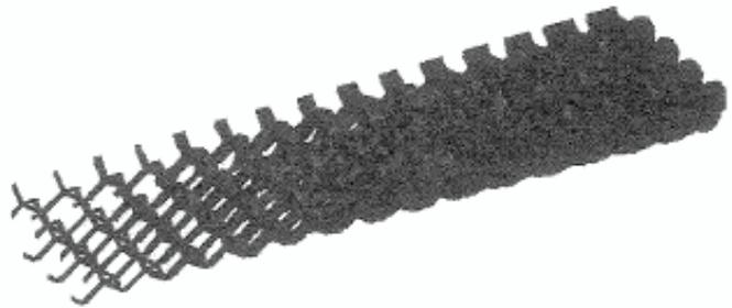
**Figure 9: Gradient TetraLattice morphology**
