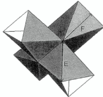
**Figure 7: Triangular TetraLattice base unit with E and F shown.**
