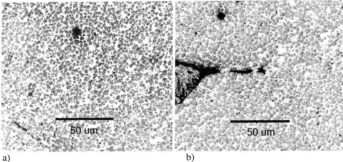
**Figure 7:** Micrograph showing a) the microstructure of extruded material and b) an interlayer region
