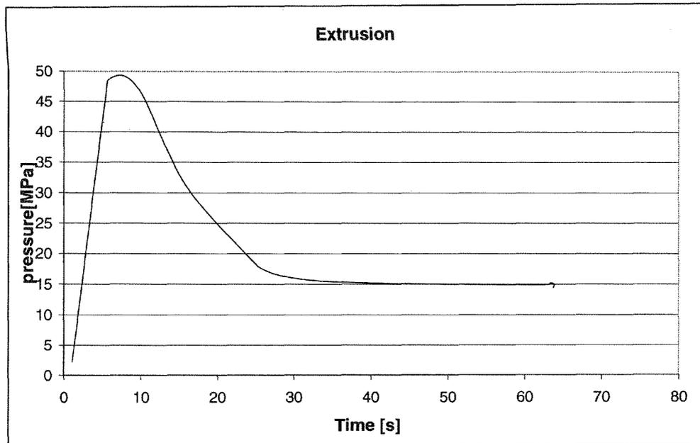
**Figure 5:** Pressure-time curve obtained from extrusion tests
