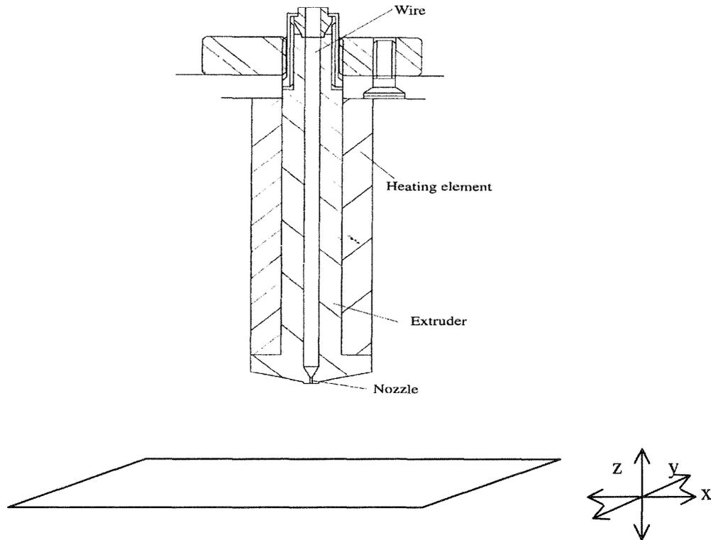
**Figure 2:** Extrusion head
