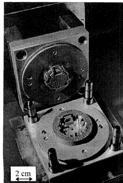
Fig. 7 Prototype tool out of 316 L, manufactured by SLPR
