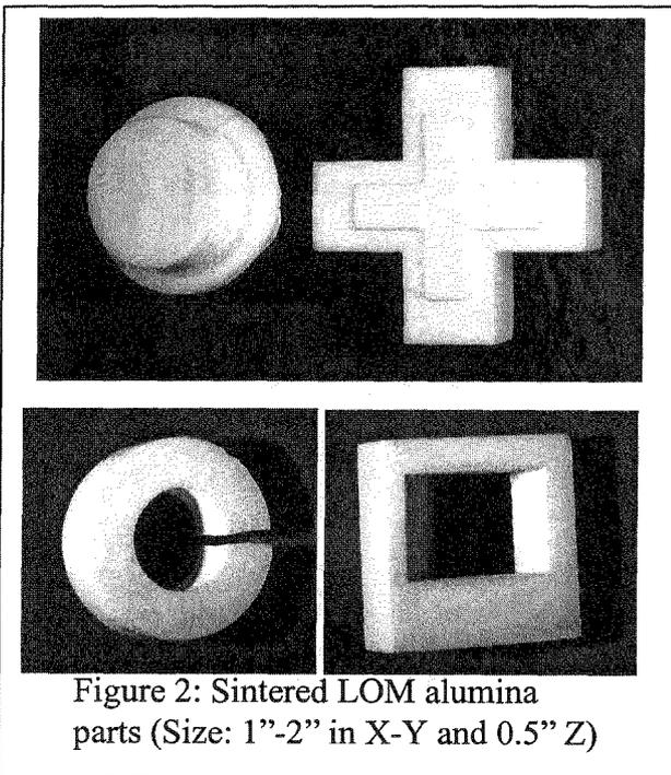
Figure 2: Sintered LOM alumina parts (Size: 1"-2" in X-Y and 0.5" Z)
