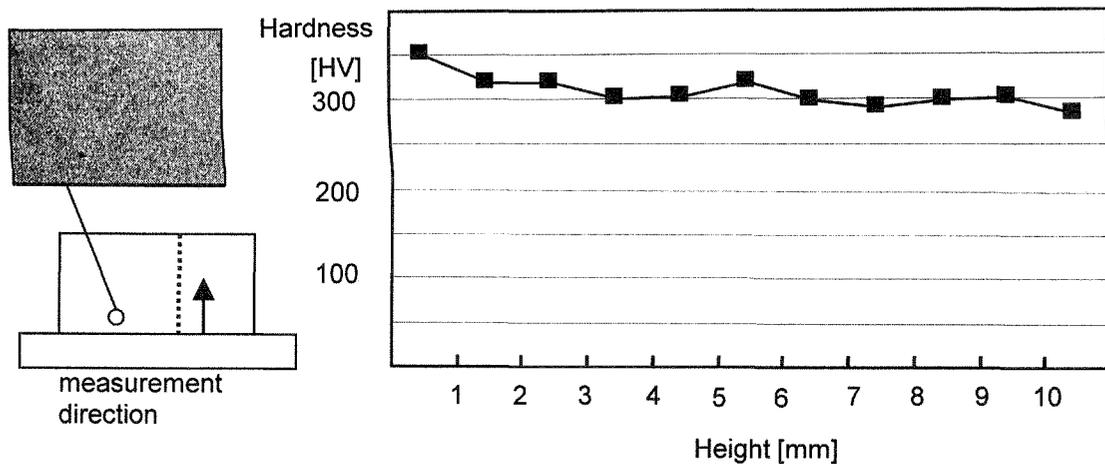
Fig. 3: Microstructure and hardness in the test specimen
