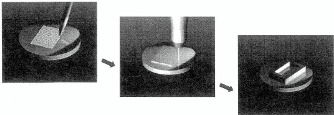
Fig. 1: Process principle of 3D Welding and Milling
