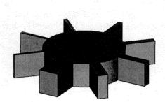
Several test parts have been designed to evaluate these properties. One is a disc with radiating arms of varying thickness. The objective of this piece is to see how thin a section can be before there is insufficient drainage of resin from the section. In addition, if the arm is too susceptible to bending there may be deformation from the desired geometry during the casting process.
