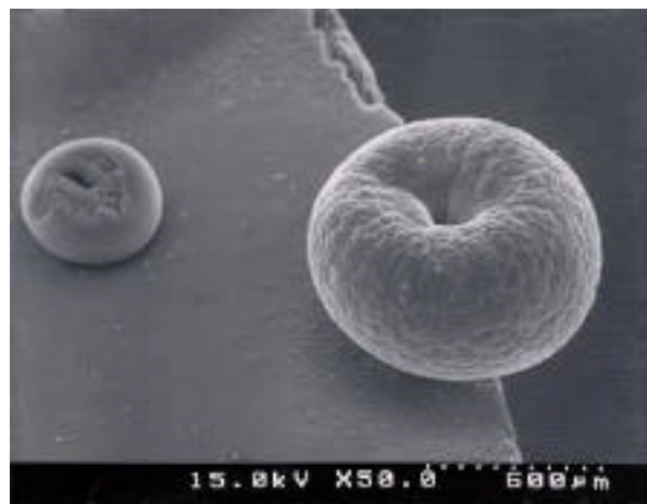
Figure 3. Both structures were deposited at 68 W of power in a static atmosphere of 75% methane and 25% hydrogen at atmospheric pressure.
