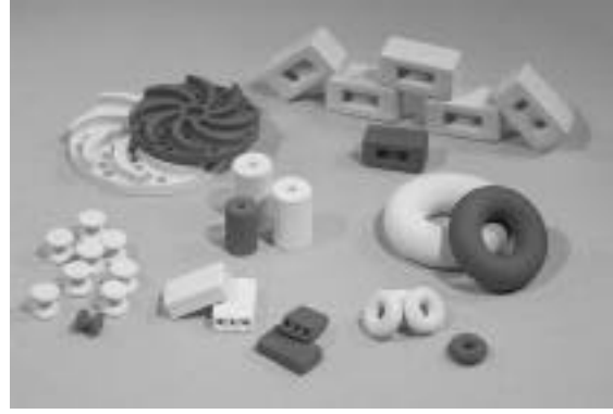
Figure 5. A set of ceramic parts made by 3D Printing. The spools in the lower left-hand corner are approximately 3mm tall.
