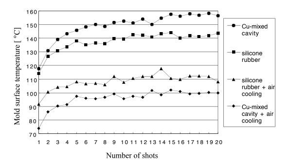
Fig.3: Surface temperatures of molds cooled with different cooling methods
