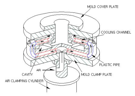
Fig. 1: Flow of cooling air through the mold
