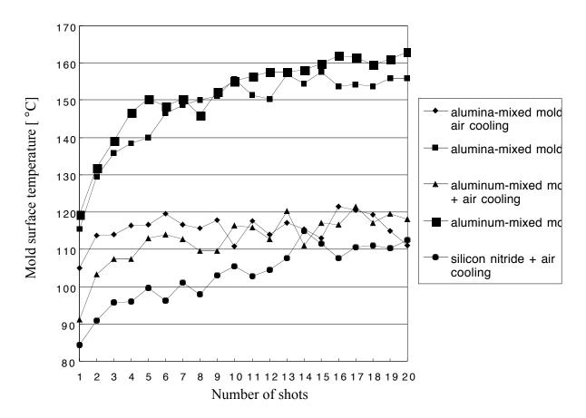
Fig. 4: Surface temperatures of molds mixed with different materials
