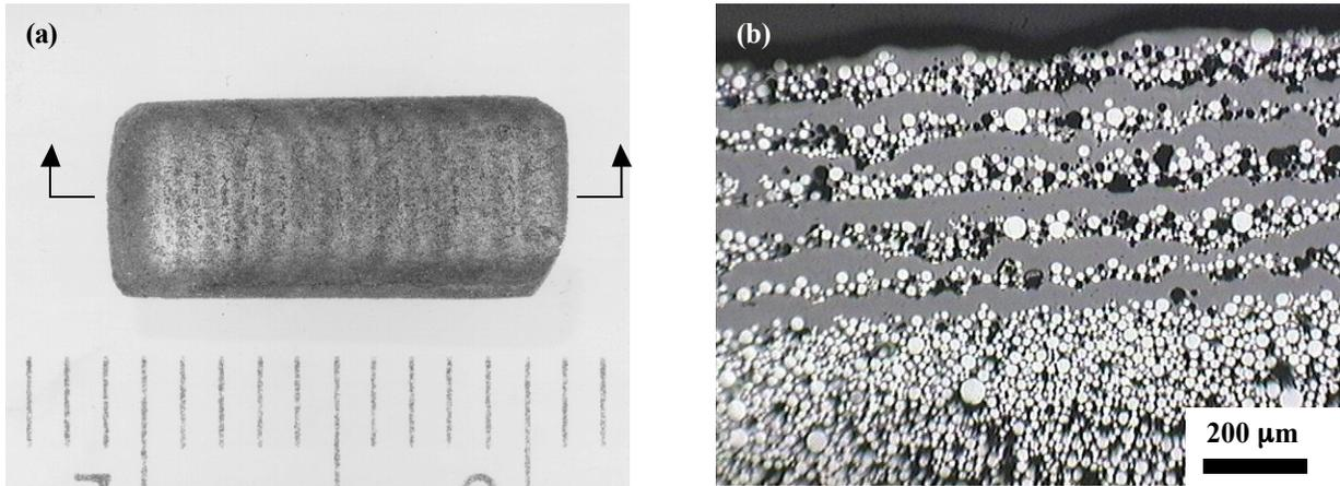
Figure 4. Mo powder/SiC matrix rectangle with 6 layers (a) as-fabricated and (b) cross-section across layers.
