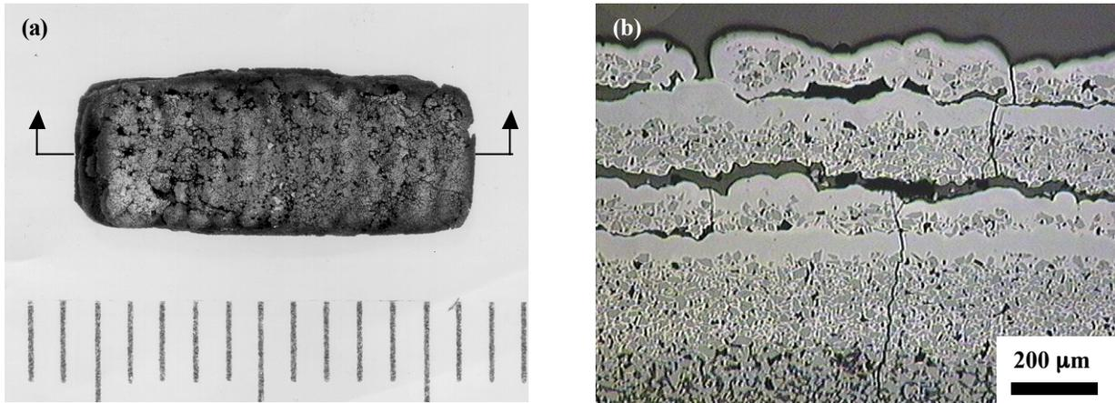
Figure 3.  $\text{ZrO}_2\text{-Y}_2\text{O}_3$  powder/SiC matrix rectangle with 4 layers (a) as-fabricated and (b) cross-section across layers.
