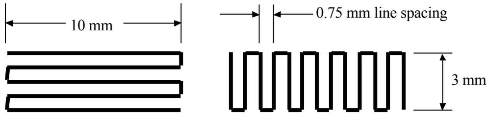
Figure 1. Scan patterns for 10 mm by 3 mm rectangle with 0.75 mm line spacing and (a) horizontal and (b) vertical major scan direction.
