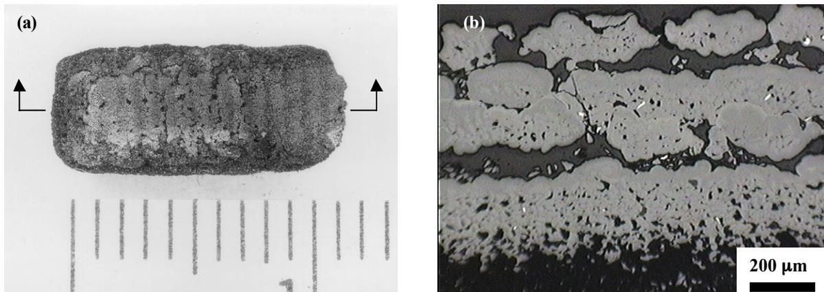
Figure 2. SiC powder/SiC matrix rectangle with 4 layers (a) as-fabricated and (b) cross-section across layers.
