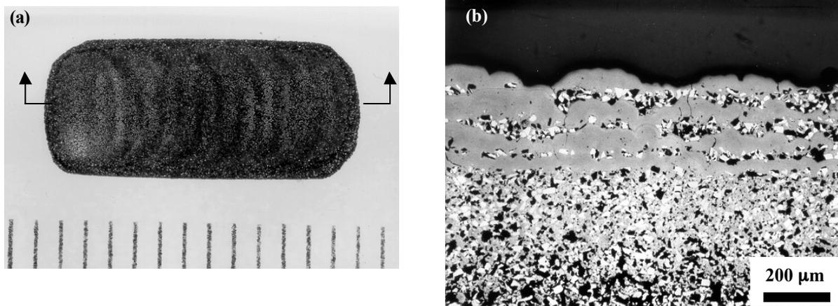
Figure 5. WC powder/SiC matrix rectangle with 4 layers (a) as-fabricated and (b) cross-section across layers.
