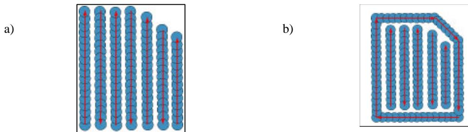
**Figure 5:** Comparison of drop placement in a) raster style and b) vector style printing<sup>3</sup>
