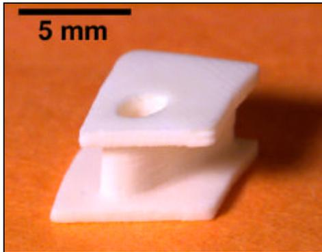
**Figure 17:** Dense Al<sub>2</sub>O<sub>3</sub> stator
