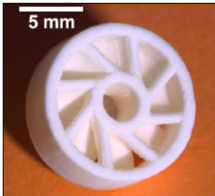
**Figure 19:** Dense Al<sub>2</sub>O<sub>3</sub> rotor
