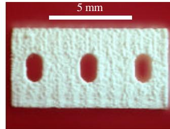
**Figure 13(a):** The front view of the S-3DP™ RF filter      **Figure 13(b):** The rear view of the S-3DP™ RF filter
