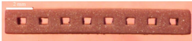
**Figure 14(a):** The front view of the S-3DP™ EBG device
