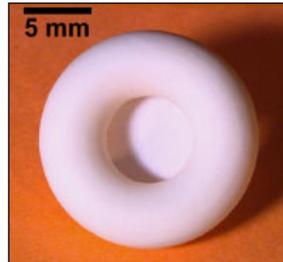
**Figure 18:** Dense Al<sub>2</sub>O<sub>3</sub> toroid
