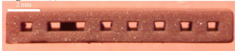
**Figure 14(b):** The rear view of the S-3DP™ EBG device
