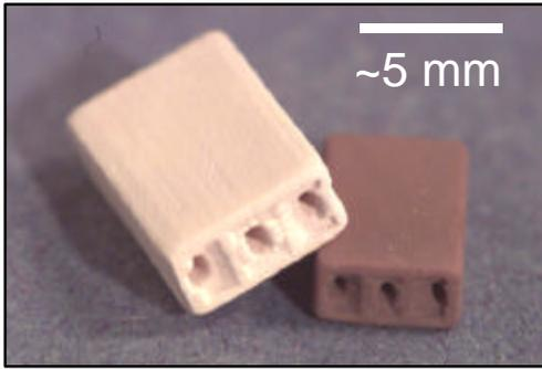
**Figure 15:** Green and dense BaTiO<sub>3</sub>-based RF filters
