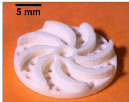
**Figure 20:** Dense Al<sub>2</sub>O<sub>3</sub> sample geometry
