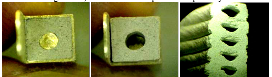
Figure 11. Laying hollow sections through CC: (a) the ceramic material in the nozzle before extrusion, (b) hollow circle formed as the extrudate emerges from the orifice, and (c) cross section of the fabricated part revealing the hollow sections
