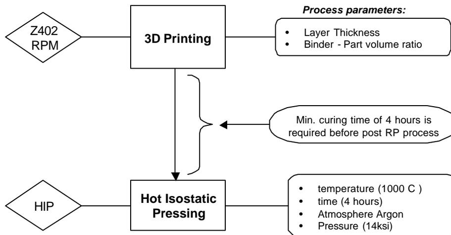
Figure 11: Flow chart of rapid prototyping of TiHA implant
