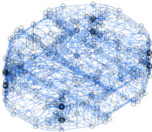
Figure 6: FEA mesh of the implant
