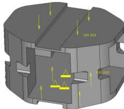
Figure 7: Constraints and loading
