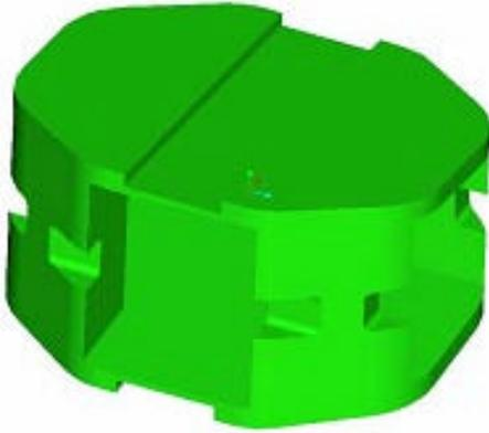
Figure 4: CAD model of the designed inter-vertebral implant
