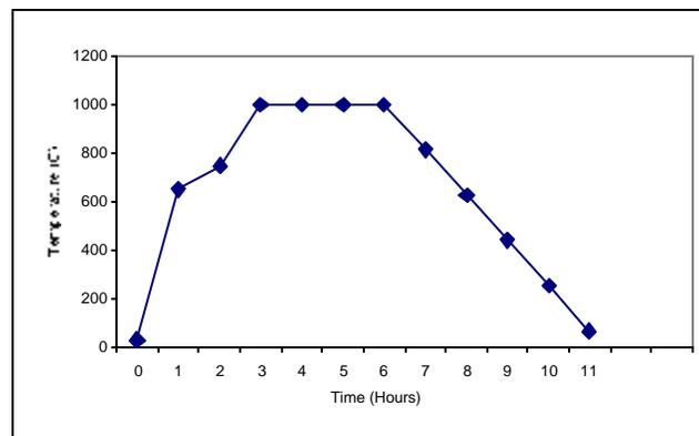
Figure 12: Temperature profile in HIP process
