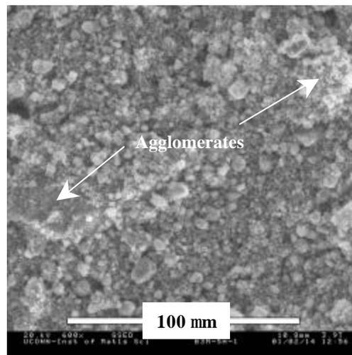
Fig. 2 ESEM image of the porcelain powder after 5 hours of dry ball milling.
