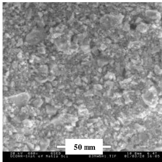
Fig. 5 Morphology of the porcelain powder after wet milling for 5 hours.
