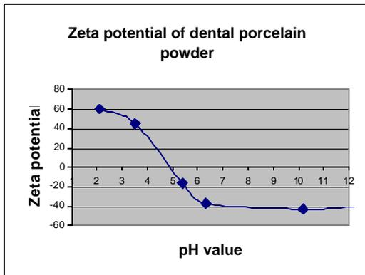
Fig. 6 Zeta potential of the dental porcelain powder as a function of pH value.
