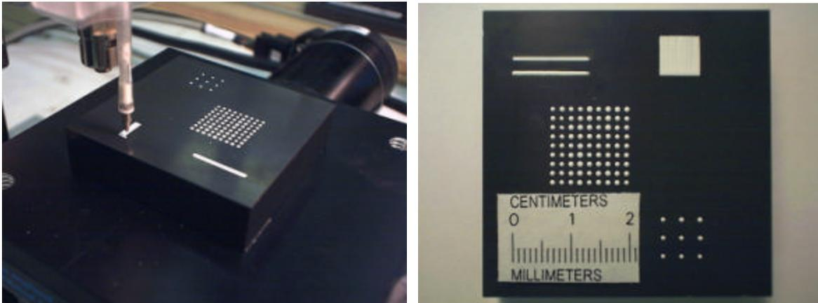
**Figure 8. (a) porcelain suspension delivery system, and (b) 2-D samples delivered.**
