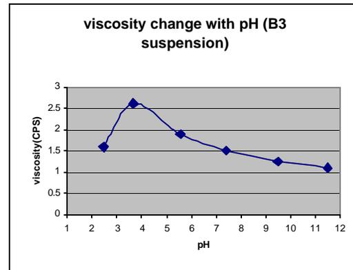
Fig. 7 Viscosity change of the porcelain suspension with pH value (8 vol% solid).
