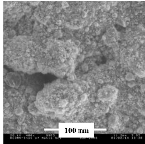
**Fig. 4** Particle agglomeration in the porcelain powder with 2 hours of dry milling.
