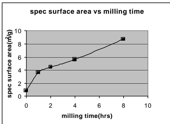
**Fig. 3** The specific surface area of the porcelain powder as a function of dry milling time.
