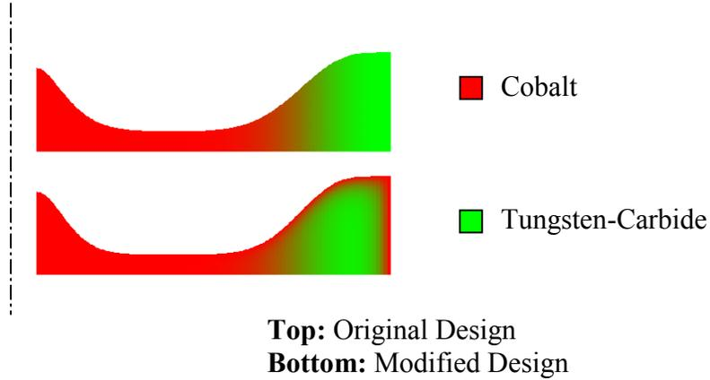
**Figure 3.** Original and Modified Flywheel Design
