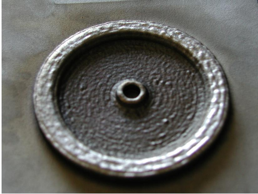
**Figure 5.** Exterior View of the Gradient Flywheel
