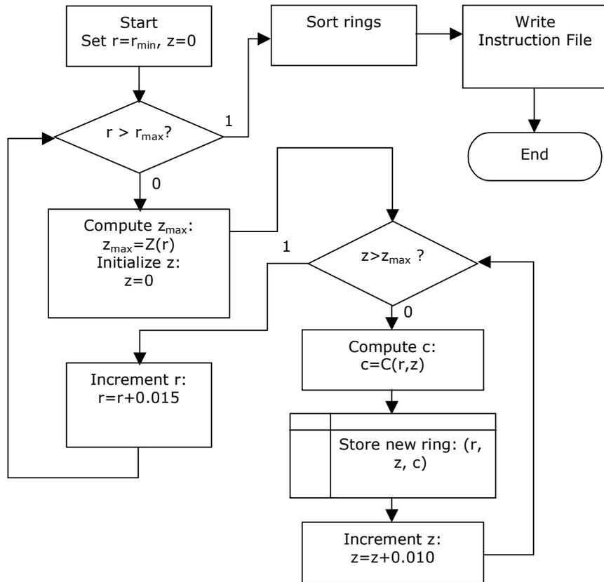
**Figure 6.** Flywheel File Preparation Flowchart
