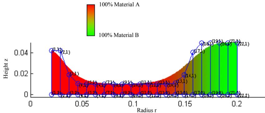
**Figure 2.** MMA-Rep of Heterogeneous Flywheel Using Bezier Interpolation
