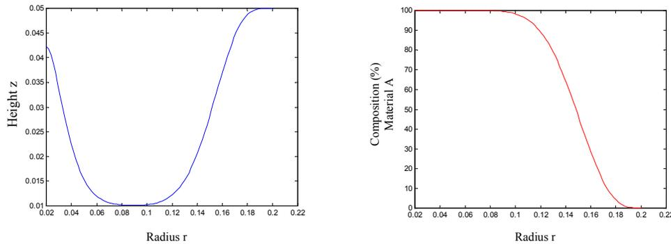
**Figure 1.** Optimal Geometry and Composition for a Heterogeneous Flywheel
