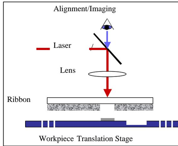
**Figure 5:** Schematic diagram of the MAPLE DW process.
