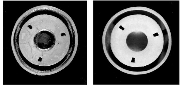
**Figure 2A and 2B:** Optical micrographs showing a bottom view of the consolidated telescoping actuators made with an unsatisfactory tape formulation (A) and a satisfactory tape formulation (B). Note that the outer cylinder diameter is 2.5 cm.
