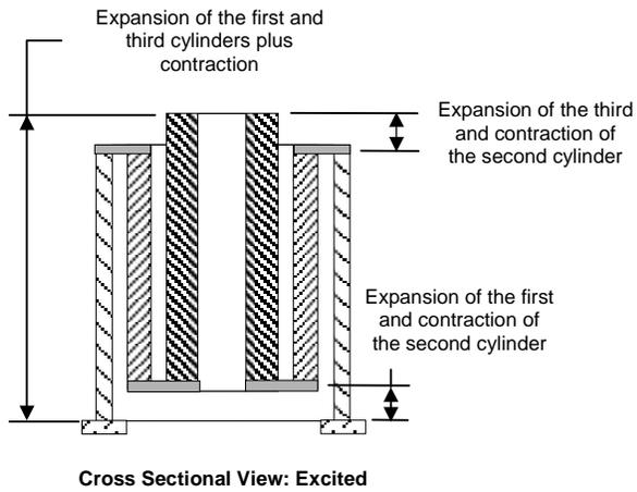
**Figure 1:** Schematic cross-sectional view of the telescoping actuator.
