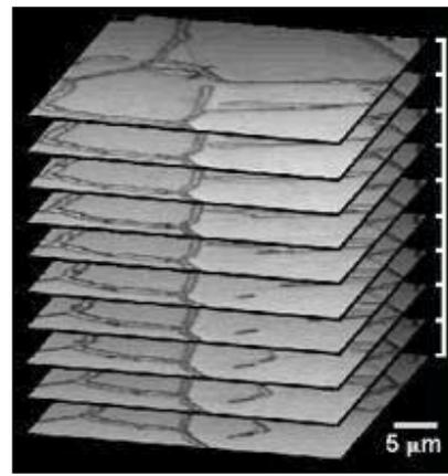
**Figure 6A and 6B:** (A) FDM model of cementite precipitates and austenite grain in a high carbon steel, and (B) a portion of the stack of 250 images of optical microstructures used as slices for the FDM process.
