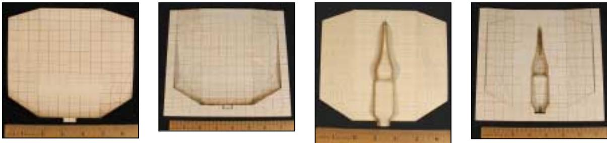
**Figure 3.** LOMS pattern and molds for a micro-air vehicle fuselage.
