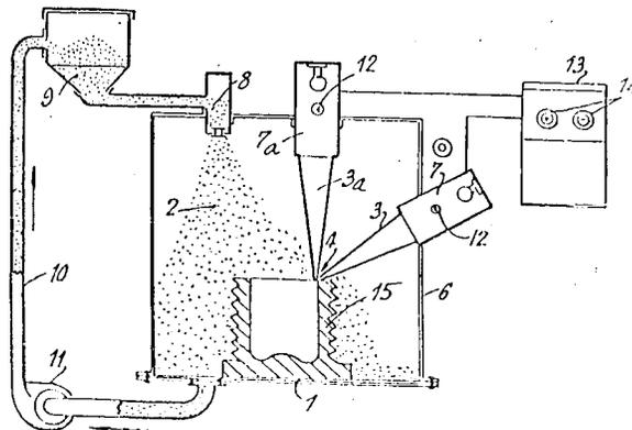
Figure 9: Powder SFF process of Ciraud.
