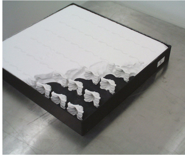
Figure 21. Bioceramic eye sockets made by 3D Printing.
