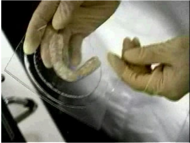
Figure 13. The aligner is made by thermoforming a plastic sheet over the stereolithography tool.
