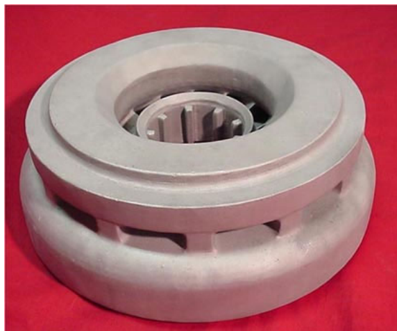
Figure 26. A ceramic mold and casting for a fuel cross over made by Soligen, Inc.
