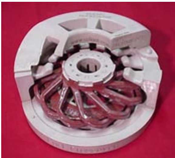
Figure 26. A ceramic mold and casting for a fuel cross over made by Soligen, Inc.
