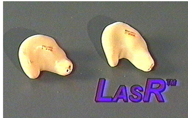
Figure 18. An SLS hearing aid is on the right while a conventionally fabricated one is on the left.
