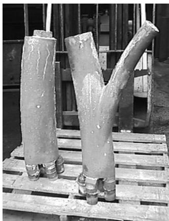
Fig. 7b. 316 Stainless prototypes, as cast and powder coated.
