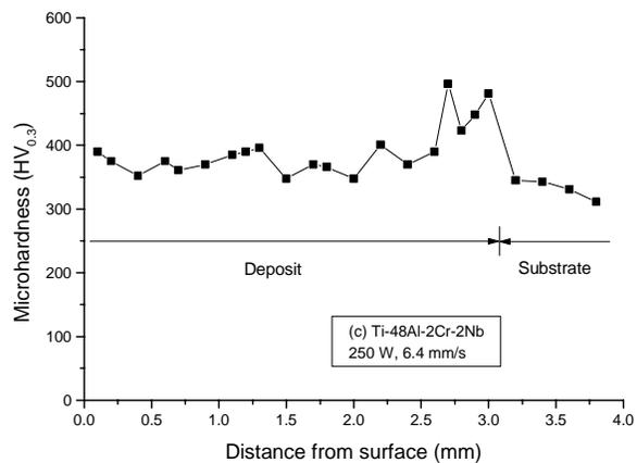
Fig. 9 Microhardness distributions: (a) and (b) the composite deposits; (c) monolithic titanium aluminide deposits.
