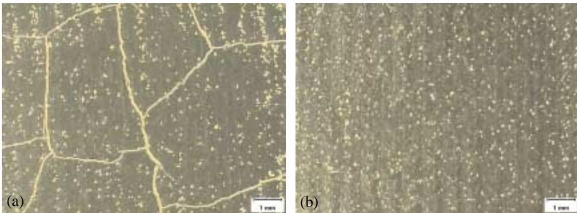
Fig. 8 Effectiveness of preventing cracking in Ti-48Al-2Cr-2Nb+TiC composite deposits by heating the substrate during processing: (a) without preheating; (b) heating to  $450^{\circ}C$ .
