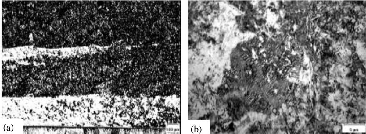
Fig. 1 Microstructure of as-deposited monolithic Ti-48Al-2Cr-2Nb alloy: (a) near the substrate; (b) massively transformed  $\gamma$  phase.
