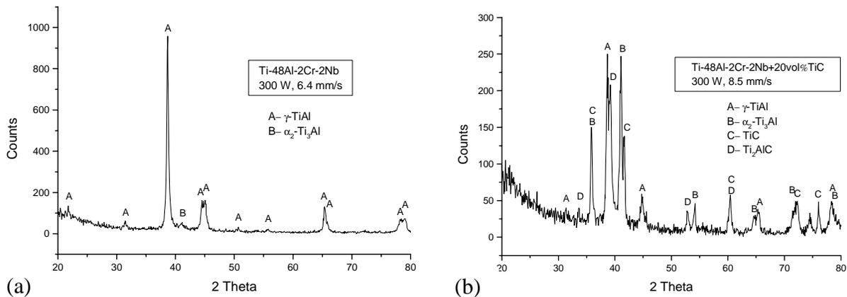
Fig. 2 X-ray diffraction patterns of LENS deposits of (a) Ti-48Al-2Cr-2Nb and (b) Ti-48Al-2Cr-2Nb+20 vol% TiC.
