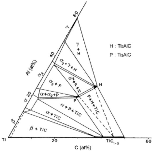
Fig. 4 A partial isothermal section of the Ti-Al-C ternary system at 1050°C [14].
