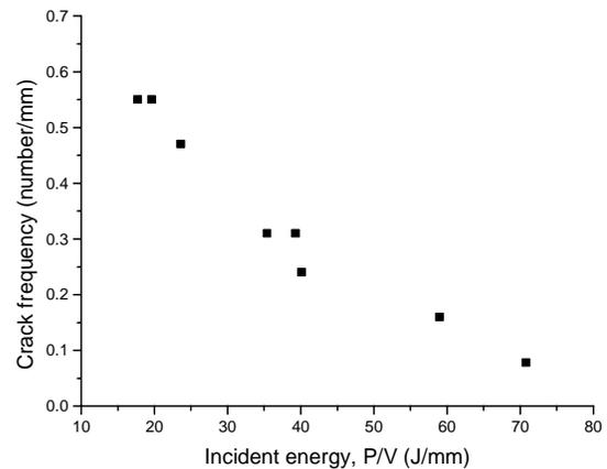
Fig. 7 Dependence of cracking frequency on the incident laser energy for the composite deposits.
