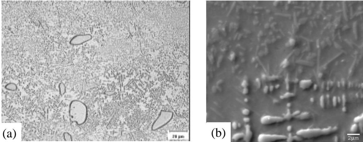
Fig. 3 Microstructure of Ti-48Al-2Cr-2Nb+20v%TiC composite deposit (as-polished) processed with a 300 W laser power and 8.5 mm/s traverse speed: (a) light micrograph; (b) SEM micrograph.
