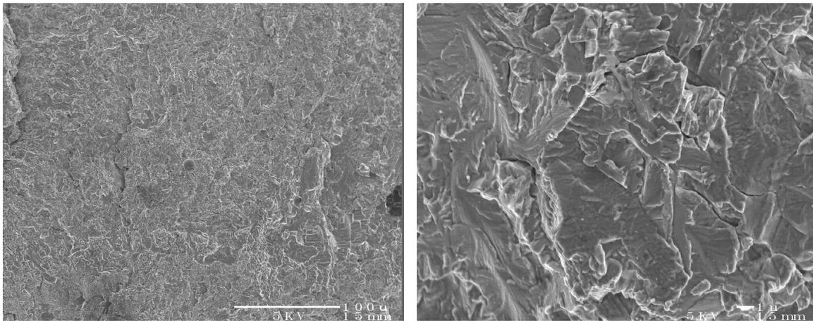
Fig. 6 SEM fractographs at different magnifications of crack surfaces observed in a Ti-48Al-2Cr-2Nb deposit (300W, 10.6 mm/s).
