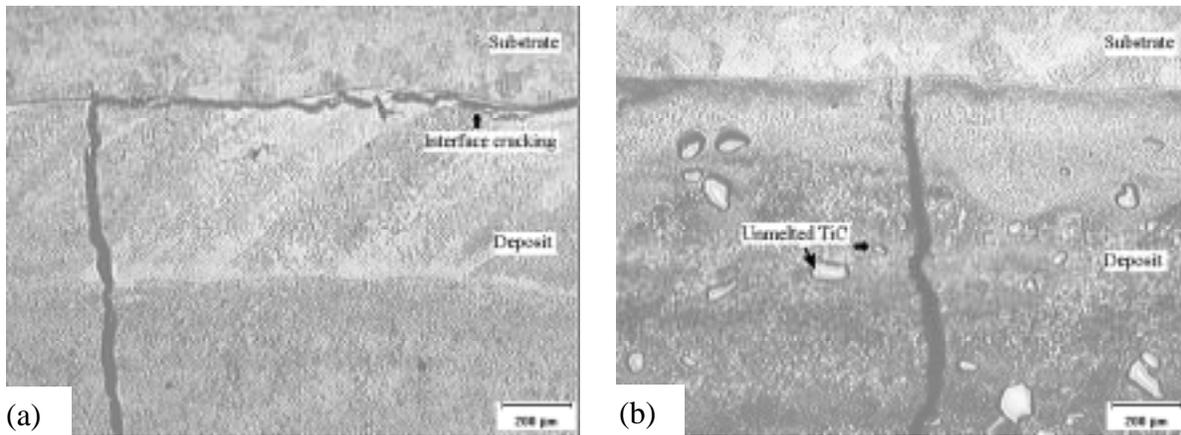
Fig. 5 Cracks observed in (a) Ti-48Al-2Cr-2Nb (300 W, 8.5 mm/s) and (b) Ti-48Al-2Cr-2Nb+20v%TiC (250 W, 6.4 mm/s) deposits.
