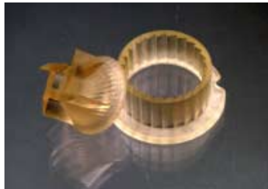
Fig. 3 Master patterns fabricated using SLA
