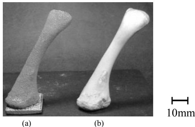
**Figure 11** – Example of a part built by selective laser melting process: (a) titanium model (b) real model
