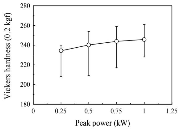
**Figure 4** – Influence of the peak power on the hardness;  $f = 50$  Hz and  $P_{av} = 50$  W
