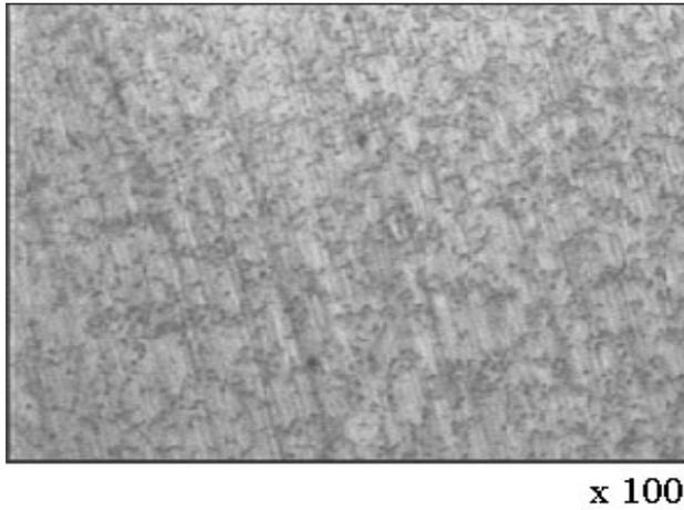
**Figure 9** – Optical micrograph after hot isostatic pressing
