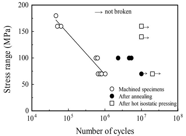
**Figure 10** – Torsional fatigue testing results after heat treatment
