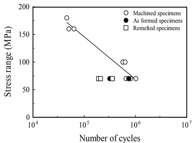
**Figure 8** – Torsional fatigue testing
