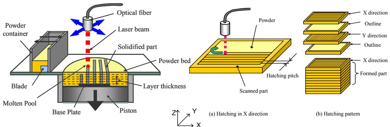
**Figure 1** – Sketch of the selective laser melting machine
