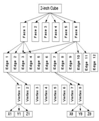
Figure 1c: Tree structure for a 2-inch cube
