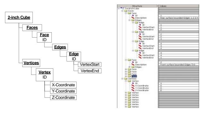
*Figure 3a: XML Structure of a 2-inch Cube*
