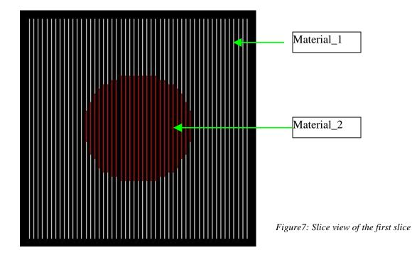
Figure 7 is a slice view displaying all the sweeps and raster segments composing the structure of the first slice. All the slicing results are stored in XML format. For example, the structure for the first sweep in the first slice can be expressed as given below. The material assigned for each geometric body will be carried over through the slicing process to the slices' data structure, from which multi-material processing instructions are generated for manufacturing.
