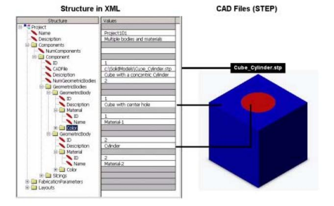
Figure 6: XML structure for fabrication of 2-body CAD model
