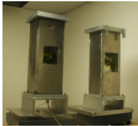
Fig 1: New powder feeders used for production of FGMs
