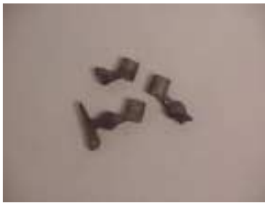
Fig. 10. Metal castings from ice patterns (Material: Talladium TILITE ceramic alloys).
