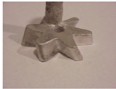
Fig. 11. Metal casting for a turbine impeller (Material: 63Sn-37Pb solder).
