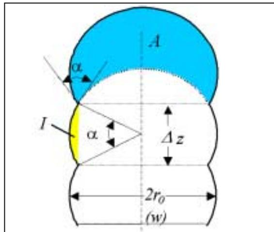
Figure 3: Cross section illustration of an ice line
