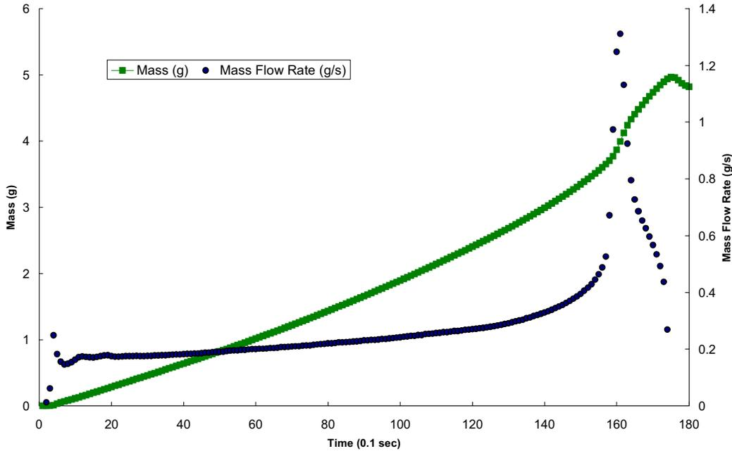
Figure 9: DuraForm PA powder delivery with no nozzle aeration pressure, radial aeration configuration, no conductive inner wall coating and no standpipe.
