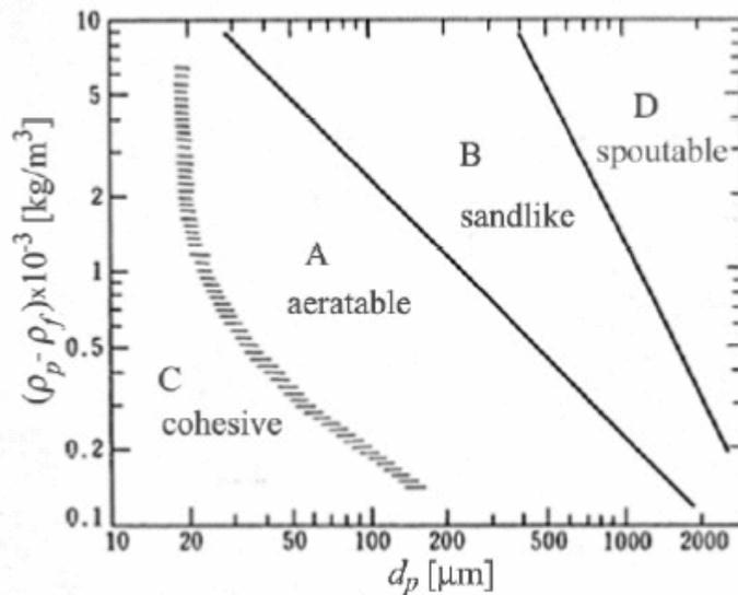
Figure 1: Geldart powder classification diagram for fluidization by air (ambient conditions) [6].
