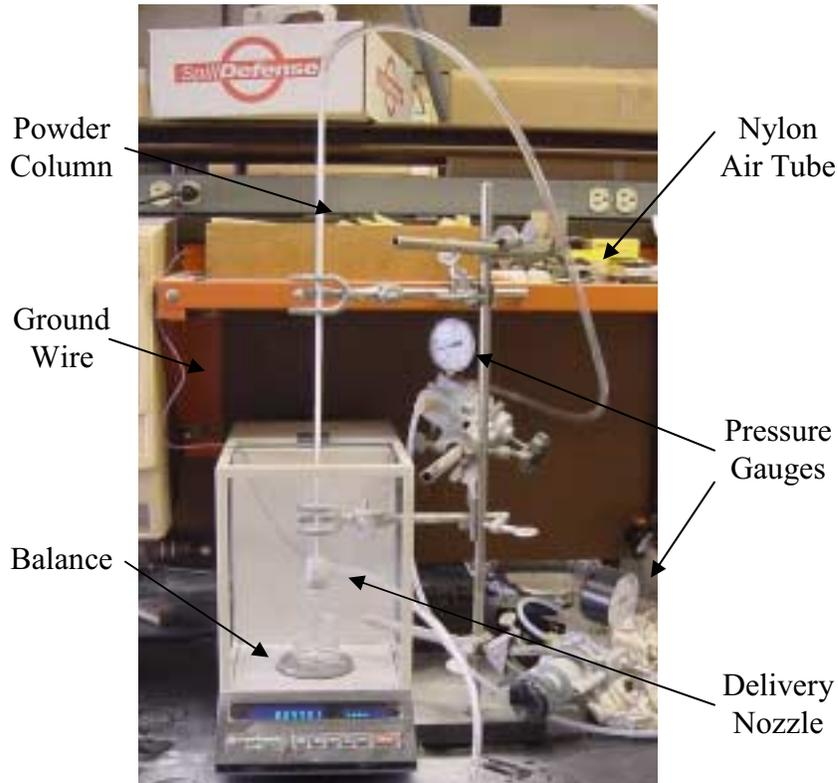
Figure 5: Experimental setup for nozzle powder delivery.
