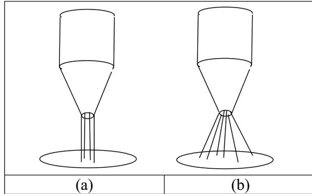
Figure 3: Powder discharge from conical nozzle (a) desired discharge with minimal spray and (b) turbulent discharge with excessive spray.
