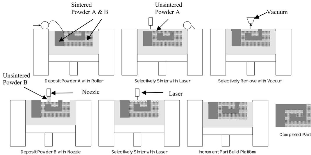
Figure 2: Schematic of precision discrete M<sup>2</sup>SLS powder delivery method.
