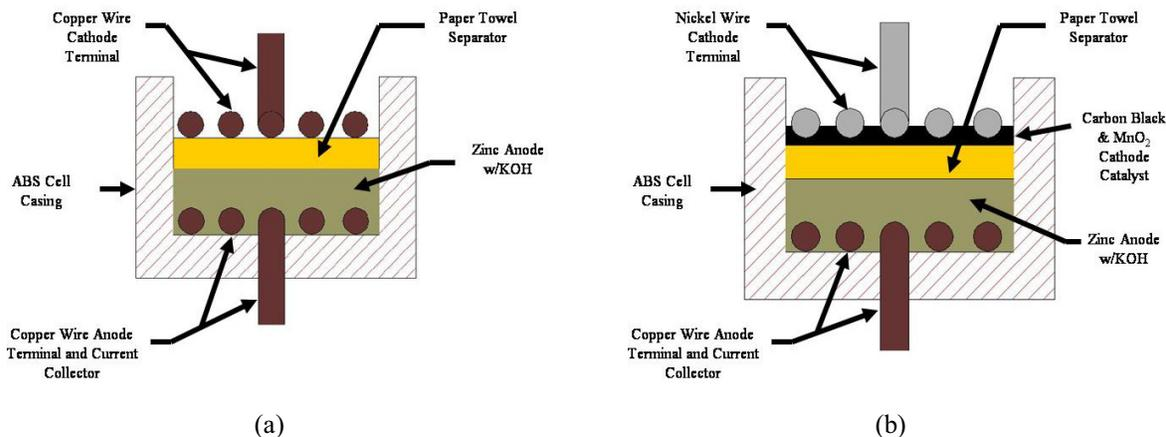
**Figure 3:** Experimental cells, in cross-section: (a) basic Zn-air cell and (b) Zn-air cell with MnO<sub>2</sub> and carbon black catalyst
