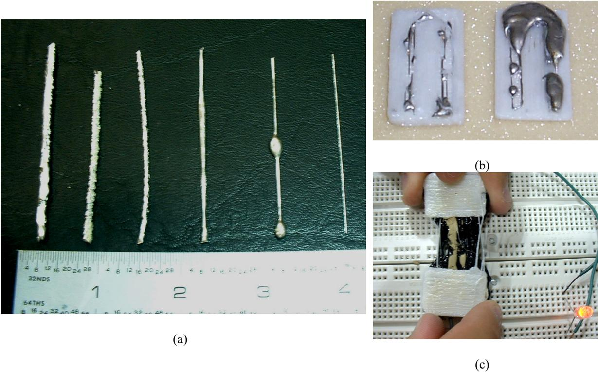
**Figure 10:** (a) Effect of deposition parameters on quality of solder alloy wiring, (b) partial success at embedding solder alloy wiring in thermoplastic part, and (c) flexure joint with silver/methylcellulose paste conductor
