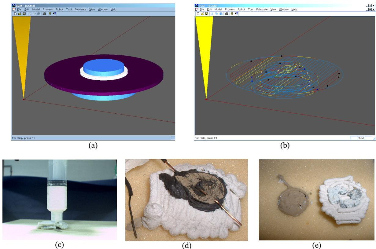
**Figure 7:** Sequence of operations in freeform fabrication of battery: (a) solid view of battery model in CCSL SCM software, (b) slicing of battery model in SCM application to generate tool paths, (c) deposition of Rescor separator layer, (d) close-up photograph of completed battery, and (e) dissection of battery (anode terminal on left and separator layer/zinc anode on right)
