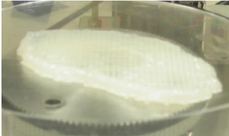
(c) Scaffold part built (15 layers)
