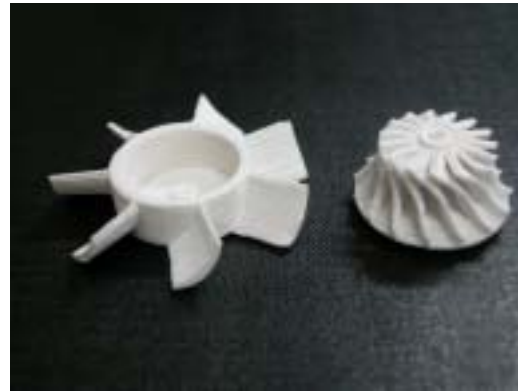
Fig. 6 Fan blade and turbine propeller made of ceramic
