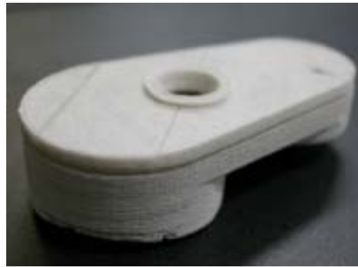
Fig. 8 A bonded CLF direct casting mold
