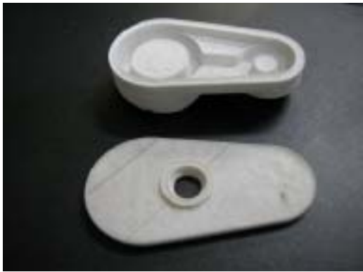
Fig. 7 A direct casting mold made by CLF
