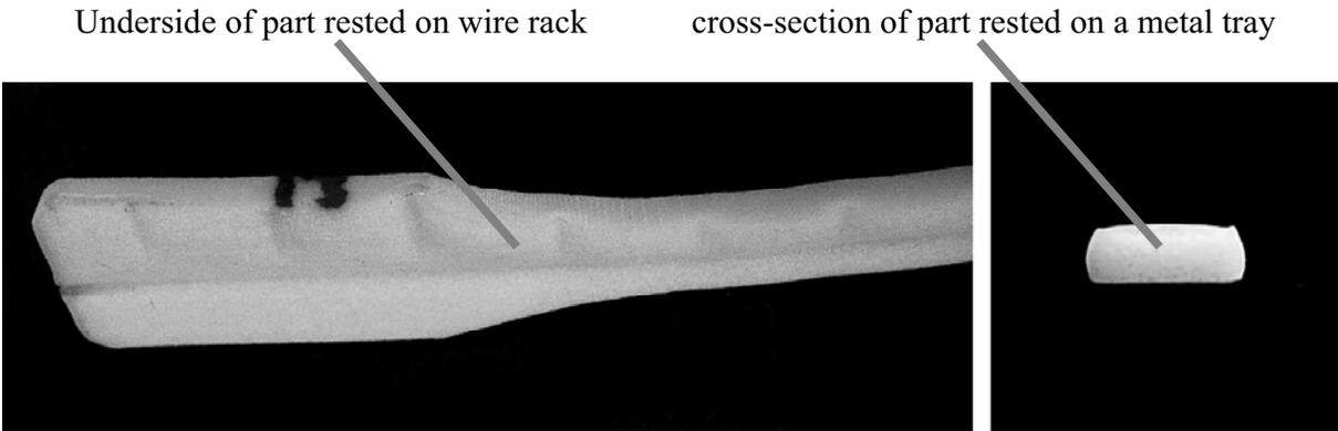
Figure 3. Deformation of parts heated to 183°C for 3 hours
