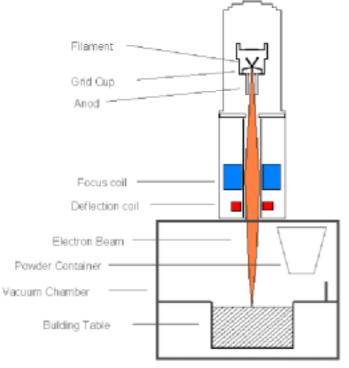
Fig. 4: Arcam EBM schematic.
