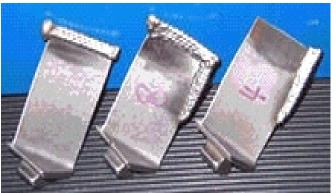
Fig. 3: Turbine blades with laser cladding build-up. (courtesy Nabil Gindy, Univ. of Nottingham)
