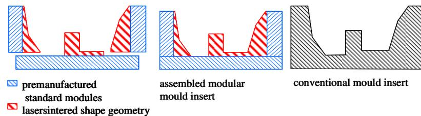
Fig. 6: Basic idea of the ecoMold project
