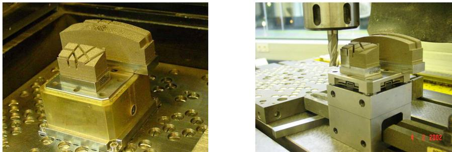
Fig. 8: Positioning system for laser sintering (left), milling and die spotting (right)
