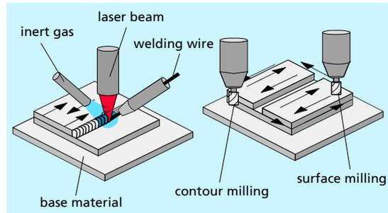
Fig. 11: Process principle of CMB
