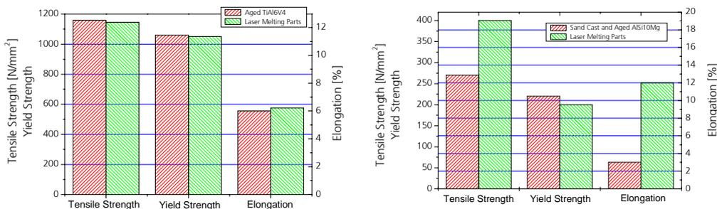
Fig. 2: Mechanical properties of TiAl6V4 (left) [3] and AlSi10Mg (right) [4] parts
