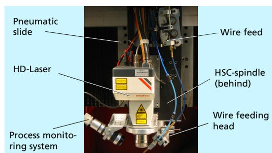
Fig. 12: CMB machine tool: High Power Diode Laser and wire feeding system
